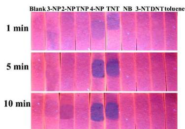
**Fig. 6.** The vapour detection of a. TNT and b. 4-NP within 1-10 min by the BSA Au-NCs test paper (concentrations of all analytes were  $10^{-4}$  M).
