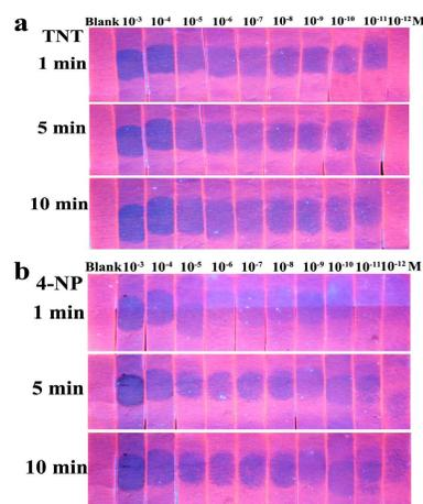
**Fig. 5.** Detection Photographs of the test strips with BSA Au-NCs under UV light, results of sensitivity of a. TNT, b. 4-NP with different reaction time.
