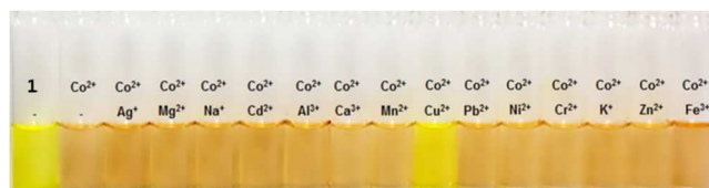
Fig. 3 (a) Competitive selectivity of 1 ( 20 \mu\text{M} ) towards \text{Co}^{2+} (0.7 equiv) in the presence of other metal ions (0.7 equiv). (b) Colorimetric changes of 1 ( 20 \mu\text{M} ) in the presence of \text{Co}^{2+} (0.7 equiv) and other metal ions (0.7 equiv).
