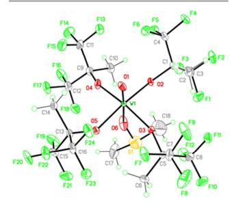
Figure 2. Displacement ellipsoid diagram of the molecular geometry of 5 with coordinated DMSO drawn at 40% probability.
