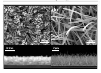
Figure 5. Plan-view and cross-sectional SEM images of materials grown from 5 at (a) 450, and (b) 550 °C.
