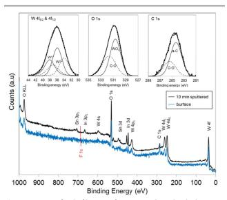
**Figure 4.** XPS scan for the film grown from **5** at 550 °C, and multiplex survey of W  $4f_5$  and  $4f_7$ , O 1s, and C 1s (Inset: Dashed lines and thin solid lines are deconvoluted peaks).
