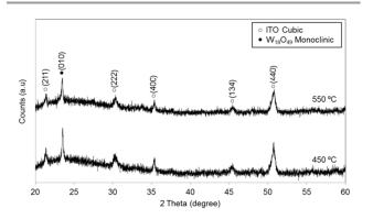
Figure 6. XRD spectra of materials grown from  ${\bf 5}$  at 450 and 550 °C.
