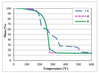
Figure 3: TGA measurements of compounds 1, 4 and 5.
