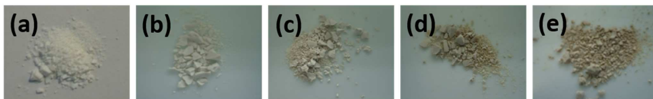
Fig. 1 Photographs showing the color change of Cu/ZIF-8 crystals upon increasing the doping percentage in copper. (a) ZIF-8 as reference, (b), (c), (d) and (e) are ZIF-8 crystals doped with 1, 5, 10 and 25% Cu, respectively.
