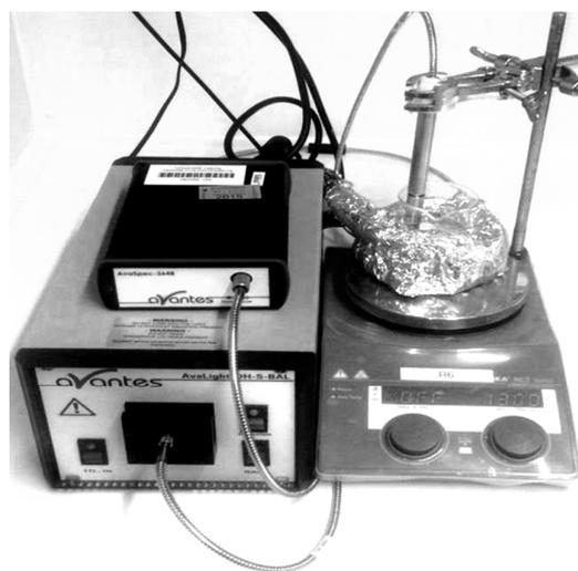
Figure 2. Experimental setup for hydrogenation of PNP with NaBH<sub>4</sub> to PAP with online UV-vis spectrometer.
