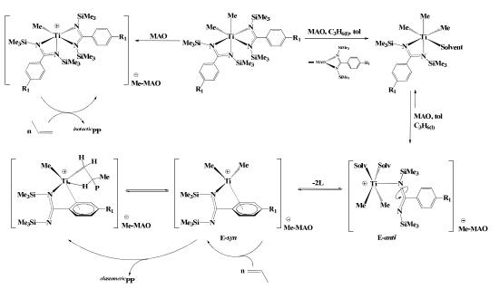
Scheme 10. Generation of active species during the polymerization of propylene with bis(benzamidinate) titanium complexes.
