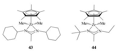
Scheme 15. Structure of the mono(amidinate) mono Cp\* complexes 43 and 44, promoting the living stereoselective polymerization of  $\alpha$ -olefins and stereo-block polypropylene.
