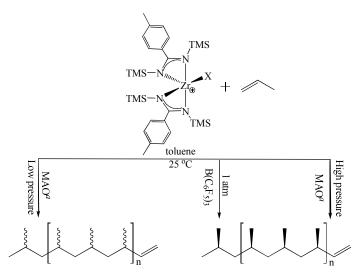
Scheme 4. Reaction conditions affecting the stereoregularity of the polymers in the polymerization of propylene. <sup>*a*</sup> different MAO ratio allows the production of the isotactic material either as the major fraction or as a mixture with an elastomeric material.
