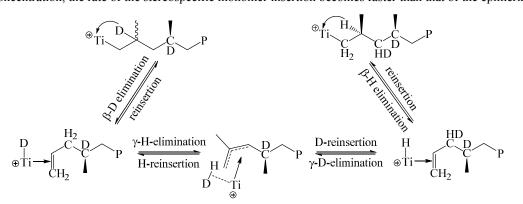
Scheme 5. Mechanistic labelling studies in the stereo-error formation in polypropylene during the reaction catalyzed by bis(amidinate) complexes.
