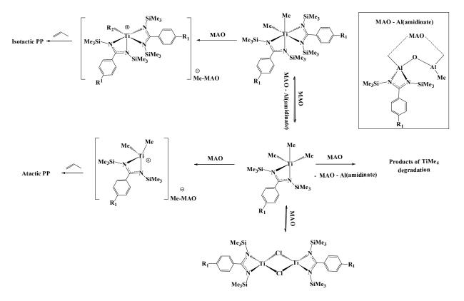
Scheme 7. Generation of active species upon the activation of titanium bis(benzamidinates) with MAO, leading to the formation of two polymeric fractions.
