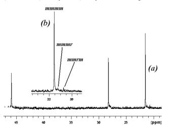
Figure 3. <sup>13</sup>C-NMR of polypropylene obtained from the catalytic mixture of **43**:MAO 1:1000 (a) full spectrum, (b) enlarged methyl region. "Reprinted with permission from T. Elkin, M. Botoshansky, R. M. Waymouth, M. S. Eisen *Organometallics*, **2014**, *33*, pp 840–843. Copyright (2014) American Chemical Society"
