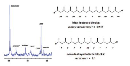
Figure 2.<sup>13</sup>C NMR spectrum of the methyl region of the hexane insoluble fraction of polypropylenes obtained by zirconium bis(amidinates). "Reproduced from Ref. 73 with permission from The Royal Society of Chemistry."
