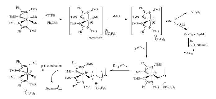
Scheme 6. Proposed mechanism for the activation of [PhC(NTMS)2]2ZrMe2 by a mixture of MAO and TTPB.
