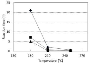
Figure 1 Reaction time needed to obtain the overall yield to PE + BPEC equal to 95% (♠), 50% (■) and 30% (♠), in function of the reaction temperature used. Reaction conditions: Phenol/ethylene carbonate 1/4 (molar ratio), catalyst/phenol 1/2 (wt ratio). Catalyst Na-mordenite SAR 13.
