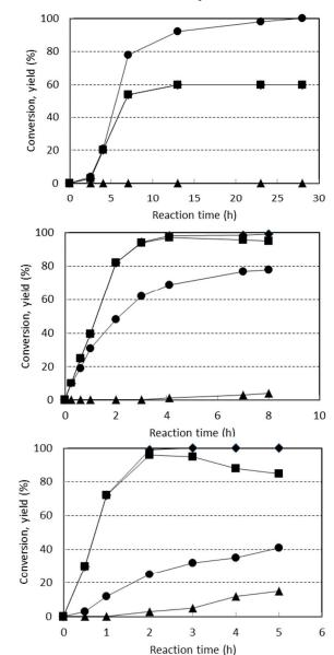
Figure 2 Effect of reaction time on phenol conversion (♠), EC conversion (♠), and yield to PE + BPEC (■), and DPE + TPE (♠). Reaction conditions: T 210°C; catalyst/phenol 1/2 wt ratio; Na-mordenite catalyst; Phenol/EC molar ratios 1/1 (top), 1/2 (middle) and 1/4 (bottom).
