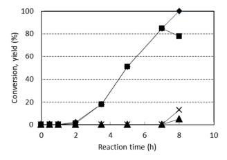
Figure 3 Effect of reaction time on phenol conversion (♠), and on yield to PE (■), BPEC (×), and DPE + TPE (♠).Reaction conditions: T 210°C, phenol/EC molar ratio 1/2, catalyst amount 0.5 wt% with respect to phenol.
