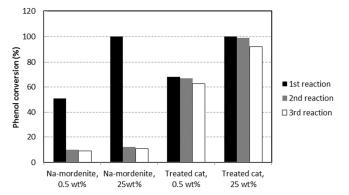
**Figure 5** Phenol conversion after 5 h reaction time at 210°C, phenol/EC ratio 1/2, with both untreated and treated Namordenite catalyst, for the fresh catalyst, and after recovery and reuse in a 2<sup>nd</sup> and 3<sup>rd</sup> reaction. Tests carried out using either 0.5 or 25 wt% catalyst (with respect to phenol).
