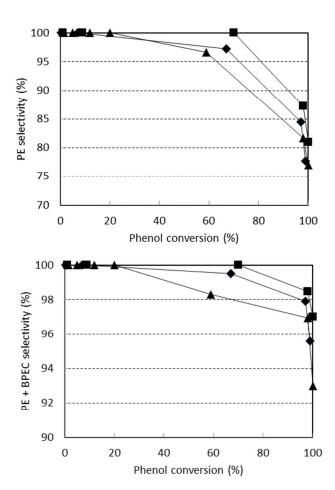
**Figure 6** Selectivity to PE (top) and to PE + BPEC (bottom) in relation to phenol conversion at  $210^{\circ}$ C, phenol/EC molar ratio 1/2, and variation of reaction time. Catalysts: treated Na-mordenite 0.5 wt% in respect to phenol ( $\spadesuit$ ), 5 wt% in respect to phenol, ( $\blacksquare$ ), and NaOH  $3\pm1$  ppm ( $\spadesuit$ ).
