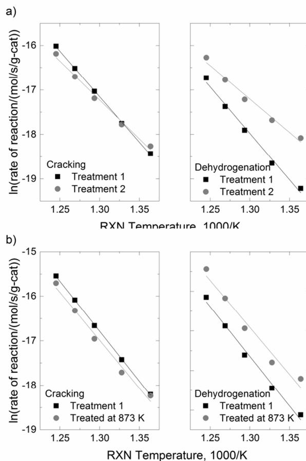
Figure 7. Log scale reaction rates for cracking and dehydrogenation of propane over a) SSZ-13-12 after the treatments 1 and 2 and b) SSZ-13-6 after treatment 1 and treated at 873 K.
