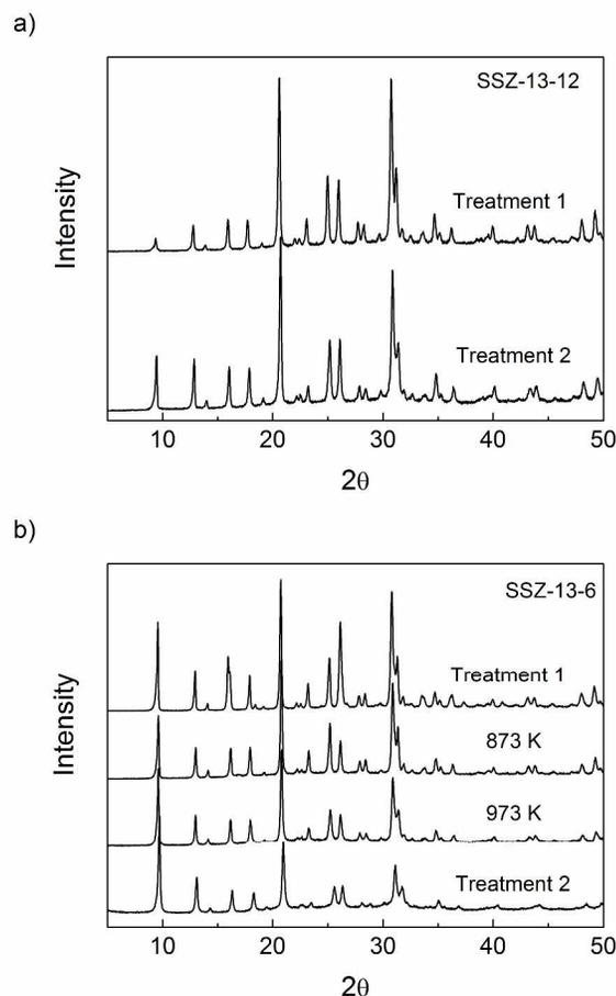
Figure 2. XRD patterns of (a) H-SSZ-13-12 and (b) H-SSZ-13-6 : calcined vs. thermally treated ones
