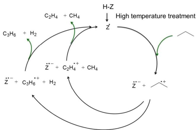
Scheme 3: Redox catalytic cycle for propane conversion over zeolite after high temperature treatment
