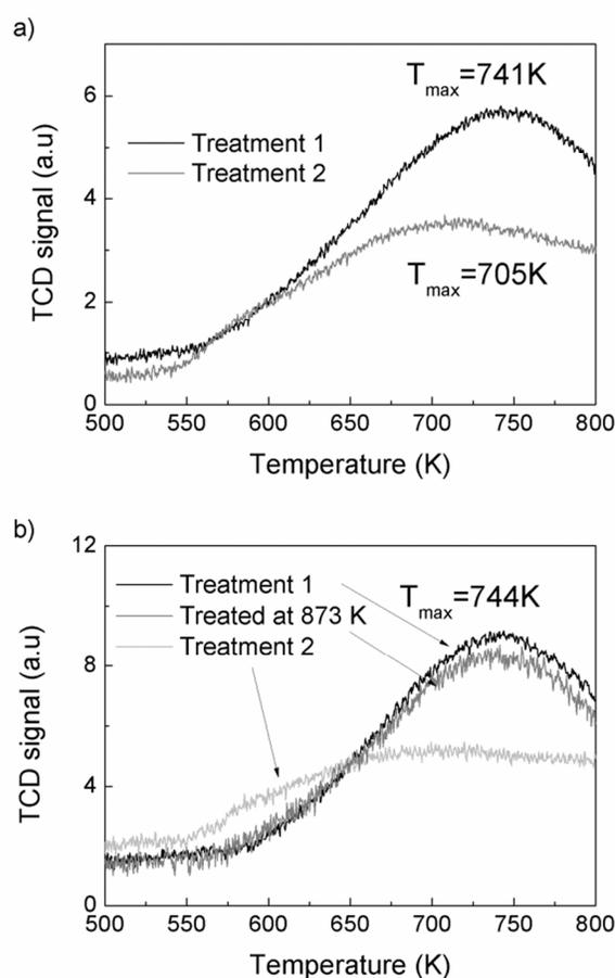
Figure 3. Ammonia TPD for (a) SSZ-13-12 after treatments 1 (black) and 2 (grey), and (b) SSZ-13-6 after treatment 1 (black), treated at 873 K (grey), and after treatment 2 (light grey)
