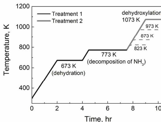
Figure 1. Temperature protocols for two treatments; 1) treatment 1 for acid catalyst and 2) treatment 2 for dehydroxylated catalyst
