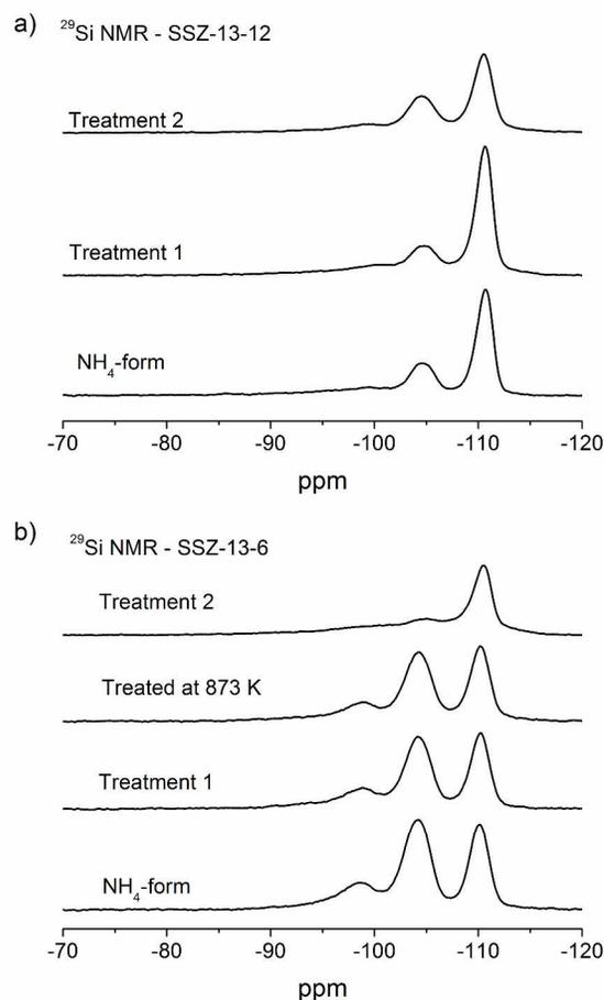
Figure 5. <sup>29</sup>Si MAS NMR of a) SSZ-13-12 samples; NH<sub>4</sub>-form, treated at 773 K and 1073 K, b) SSZ-13-6 samples; NH<sub>4</sub>-form, treated at 773 K, 873 K, and 1073 K.
