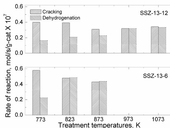
Figure 6. Reaction rates for cracking and dehydrogenation of propane at reaction temperature 773 K over SSZ-13-12 and SSZ-13-6 treated at different pretreatment temperatures.
