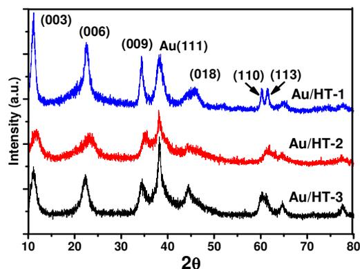
Figure 1. XRD diffraction patterns of the prepared catalysts
