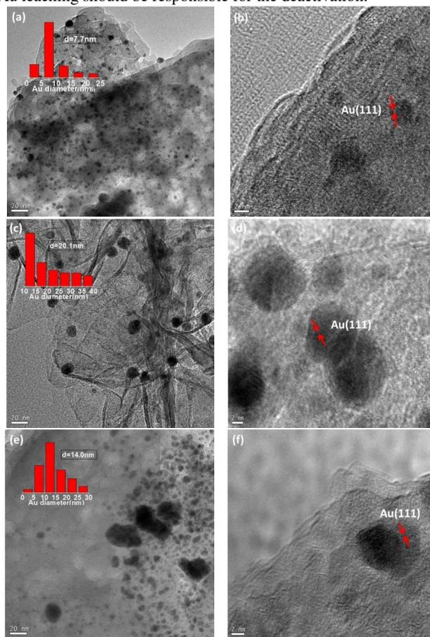
Figure 3. TEM pictures of the prepared catalysts Au/HT-1 (a, b), Au/HT-2 (c, d) and Au/HT-3 (e, f)
