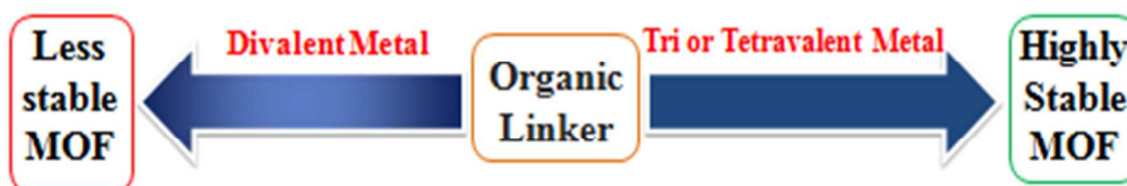
Fig. 34 Representation of the stability of MOFs prepared from different metal ions (di, tri and tetravalent).
