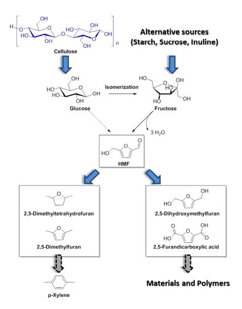
**Scheme 4.** Schematic HMF synthesis and derivatization in into useful building blocks and fuel additives.
