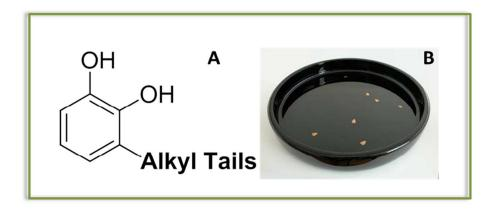
**Figure 8.** General structure of urushiol (A) and an example of lacquerware (B). Allowance request in process.
