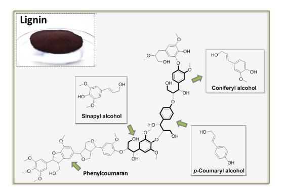
Figure 5. Schematic representation of lignin and its constituting building blocks
