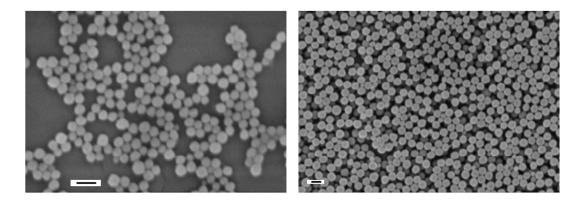
Figure 3. Scanning electron micrographs of PMGVL latexes prepared with KPS (PDL, left) and AIBN (ADL, right); the bars indicate 200 nm.
