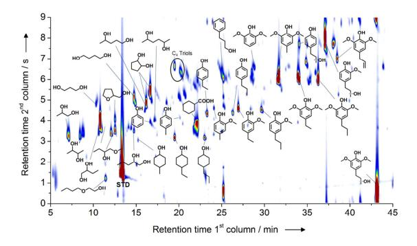
**Figure 7.** Speciation of the products obtained from the catalytic biorefining of poplar wood in the presence of Raney Ni at 1808C for 3 h (2-PrOH/H2O, 7:3, v/v). Reproduced with permission from ref. 35. Copyright 2014, Wiley-VCH Verlag GmbH & Co. KGaA, Weinheim.
