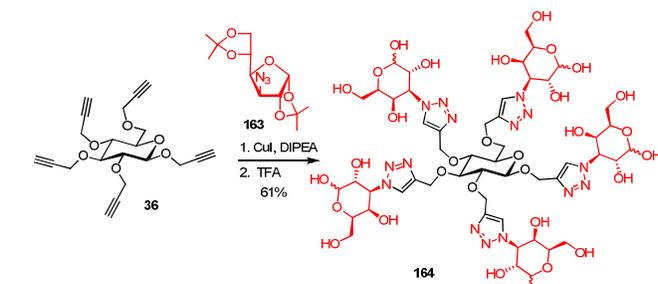
**Fig. 27** CuAAC attachment of an azido furanose derivative (**163**) onto a pentapropargylated (**36**) glucoside scaffold affording 20-OHs groups at the G1 level.
