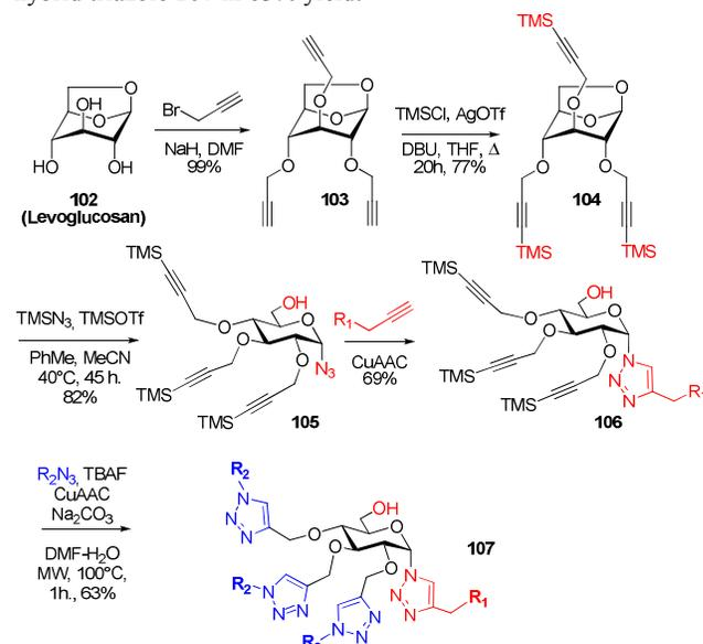
**Fig. 20.** Orthogonally-protected A<sub>3</sub>BC azido-TMS-protected alkyne involving versatile levoglucosan (**102**) as a source of glucoside 2,3,4-triol.
