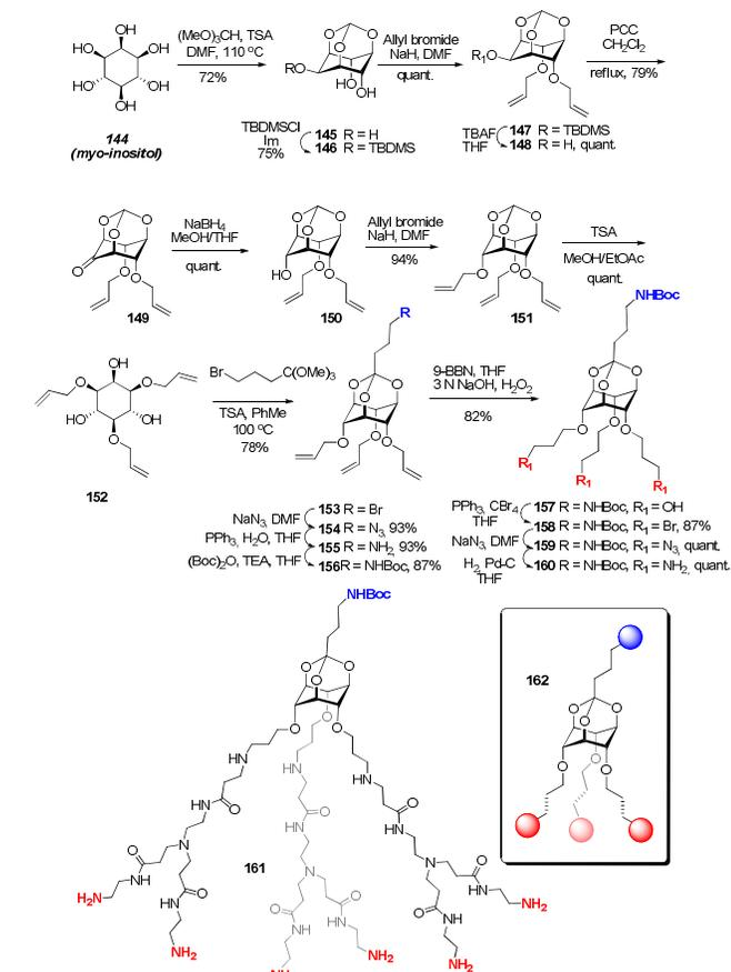
**Fig. 26** Synthetic sequence leading to a PAMAM-type symmetrical A<sub>3</sub>B scaffold starting from readily available *myo*-inositol.
