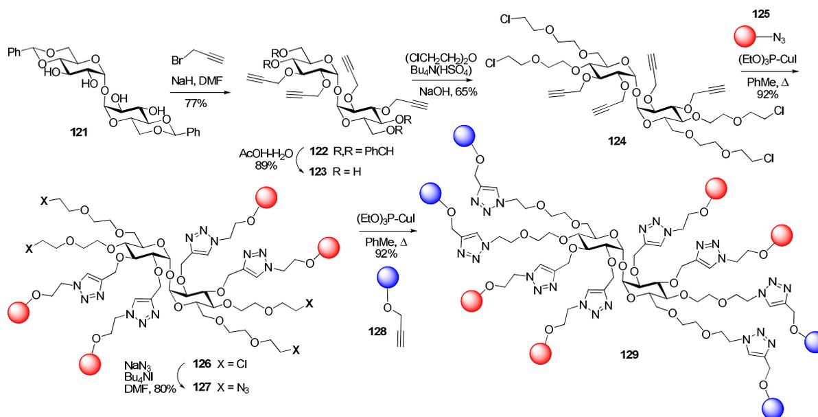
Fig. 23 Examples of orthogonally functionalized trehaloside disaccharide that can undergo regioselective CuAAC coupling.
