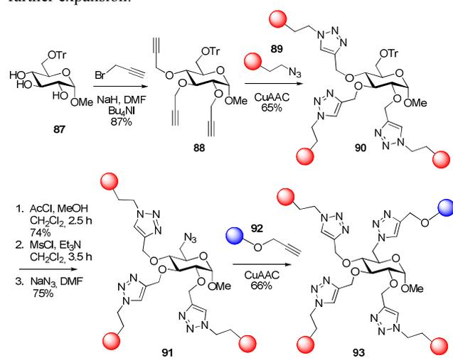
**Fig. 18** Multichromophoric sugar for fluorescence photoswitching. Red balls represent dicyanomethylenepyran fluorophores (DCM) while the
