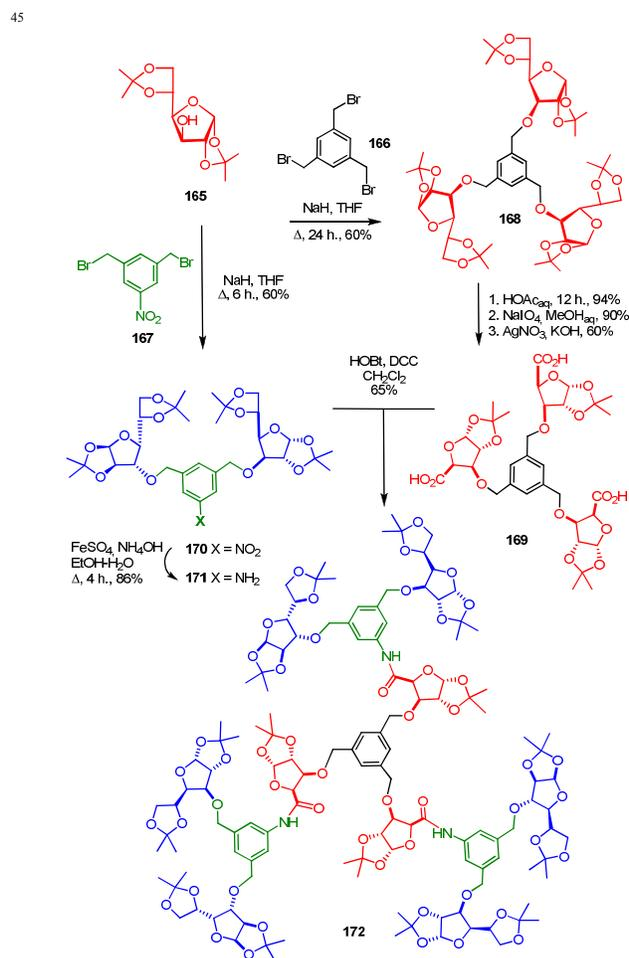
**Fig. 28** Convergent synthesis of chiral dendrimers using sugar residues.
