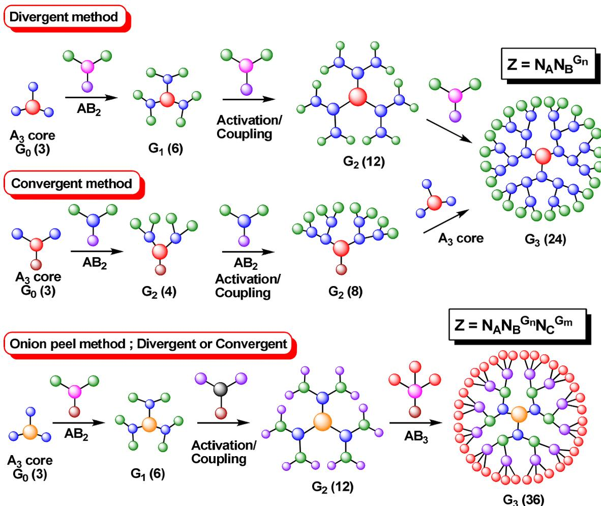
Fig. 1 Schematic representation of common strategies used to build dendrimers including the novel “onion peel” approach that allows faster surface group increase together with bringing biophysical versatility in between dendrimer generations. Numbers in parentheses refer to those of the functional groups at the periphery.
