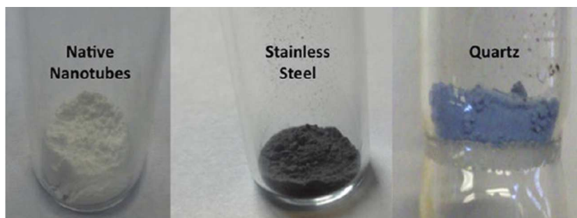
Figure 10. Pictures of titanate nanotubes and after hydrogenation at 350 °C for 3 h under a flow of 5% H 2 in Ar at atmospheric pressure in a stainless reactor and a quartz reactor. 127 Reprinted with permission from ref 127. Copyright 2012, American Chemical Society.
