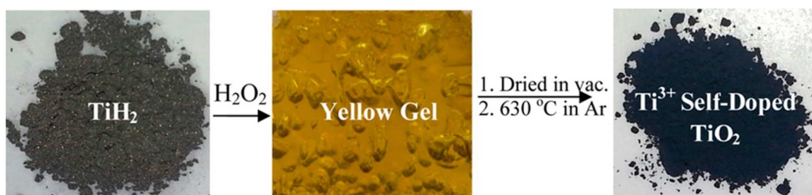
Figure 20. Illustration of the synthesis strategy from TiO 2 to black TiO 2 nanoparticles, along with their images. 152 Reprinted with permission from ref 152. Copyright 2013, American Chemical Society.
