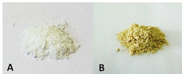
Figure 8. Pictures of anatase \text{TiO}_2 before (A) and after (B) hydrogenation for 7 h at 450 °C under a 5% \text{H}_2 / 95% Ar gas flow. 123 Reprinted with permission from ref 123. Copyright 2012, American Chemical Society.
