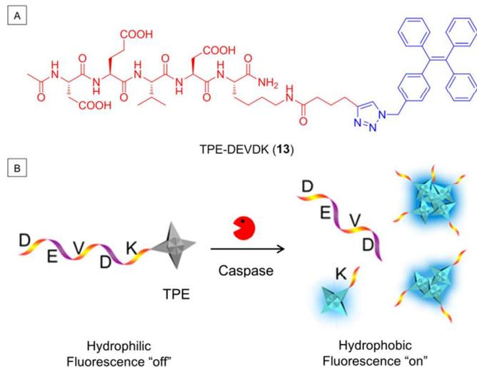
**Figure 7.** Schematic illustration of TPE-DEVDK (**13**) for caspase activity study based on the change in hydrophilic-hydrophobic property. Adopted with permission from ref. 24. Copyright 2012, American Chemical Society.
