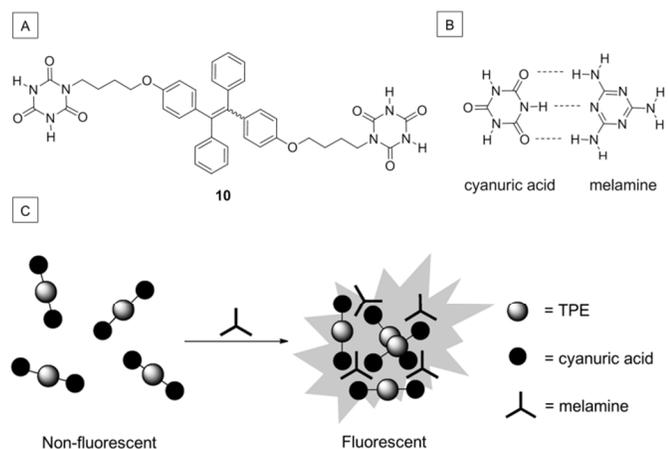
**Figure 5.** (A) The chemical structure of **10**. (B) Melamine–cyanuric acid adduct formed through multivalent hydrogen bonding. (C) The design principle of fluorescent “turn-on” sensor for melamine based on the formation of hydrogen bonds between melamine and **10**. Adopted with permission from ref. 21. Copyright 2012 Wiley-VCH.
