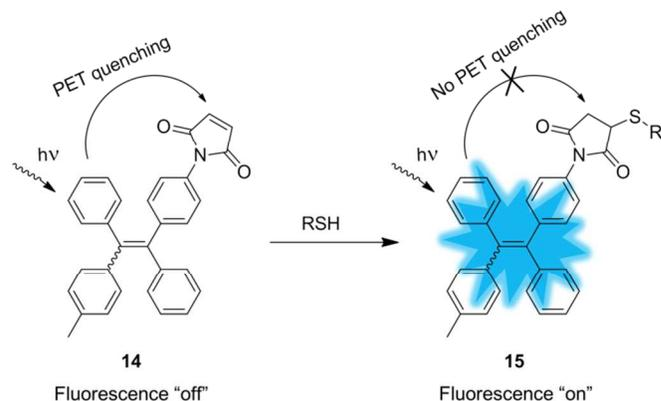
**Figure 8.** The design principle of fluorescent “turn on” biosensor **14** for thiol detection based on photoinduced electron transfer (PET) process. Adopted with permission from ref. 25. Copyright 2010 Wiley-VCH.
