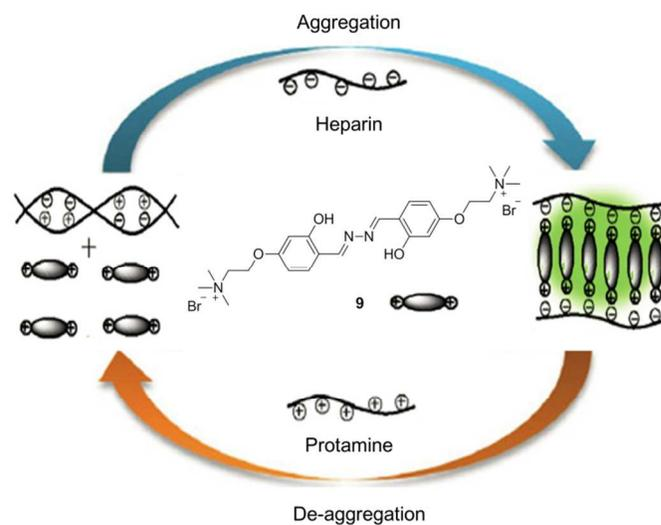
**Figure 4.** The design principle of fluorescent turn-on sensor for heparin and turn-off sensor for protamine based on aggregation and deaggregation of **9** via electrostatic attraction. Adopted with permission from ref. 20. Copyright 2013 Elsevier B.V..
