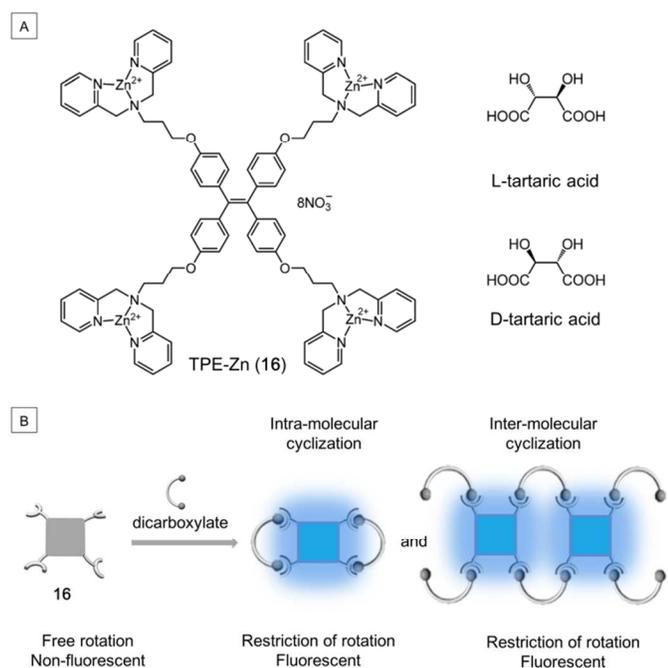
**Figure 9.** (A) Chemical structures of TPE-Zn (**16**) and chiral tartaric acids. (B) The design principle of fluorescent turn-on sensor for dicarboxylate detection based on cyclization mechanism. Adopted with permission from ref. 26. Copyright 2014 Wiley-VCH.
