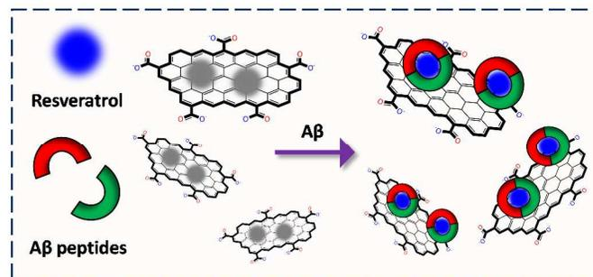
**Figure 6** Detection of Aβ peptides using resveratrol-confined GO.
