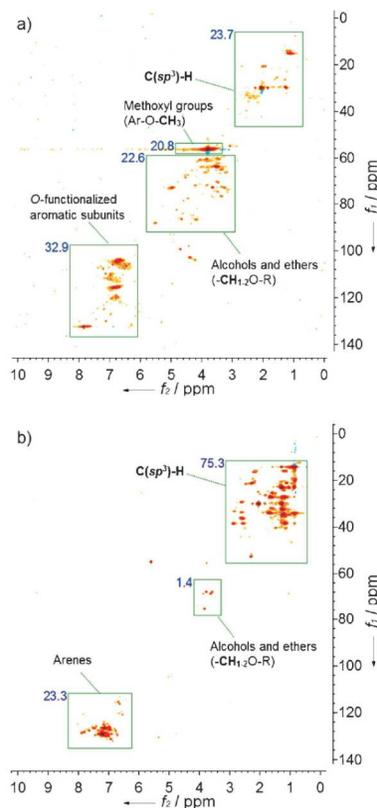
Figure 2. Catalytic tandem reaction between a phenol and 2-propanol in the presence of a reducing reagent (Raney-Ni) and oxidant (HBEA-35). The protocol was able to form mostly arenes, alkanes, and phenols. HSQC 2D NMR experiments were able to provide insights into lignin products as compared to parent organosolv lignin. Copyright by Wiley-VCH Verlag GmbH & Co.KGAA. Reproduced with permission from reference 34.
