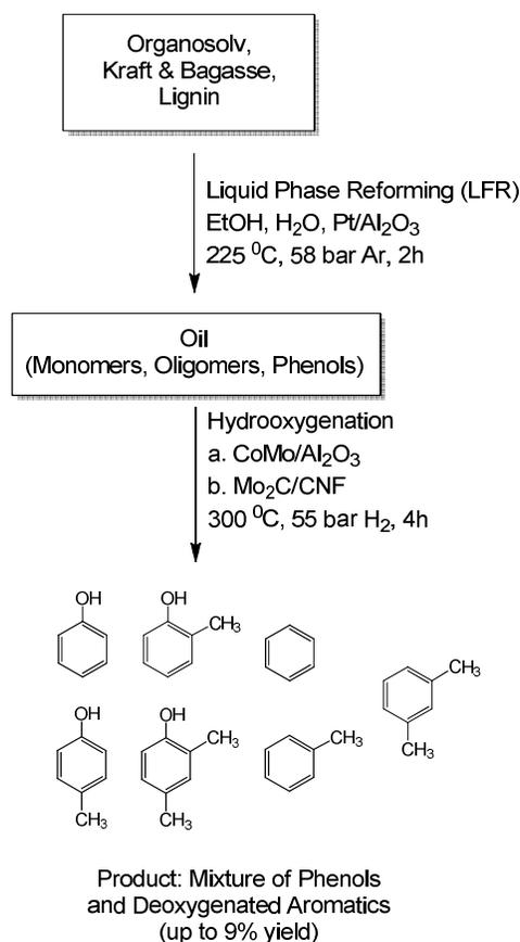
Scheme 15. Novel lignin depolymerization method involving a two-step recovery of phenolic and deoxygenated aromatic compounds.<sup>40</sup>
