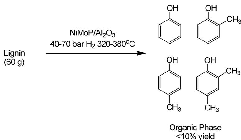
Scheme 13. Depolymerization of lignin materials using Nickel/Aluminum catalysts forming phenolic compounds in <10% yields.<sup>36</sup>
