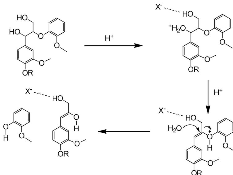
Scheme 10. Mechanism of lignin depolymerisation under acidic conditions showing the effect of IL anions.
