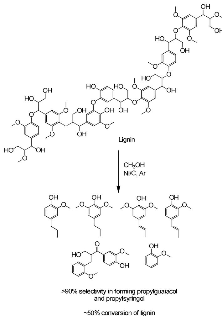
Scheme 12. Valorization of wood lignin using a Ni-based catalyst with methanol as a hydrogen solvent, selectively forming phenolic aromatic compounds.
