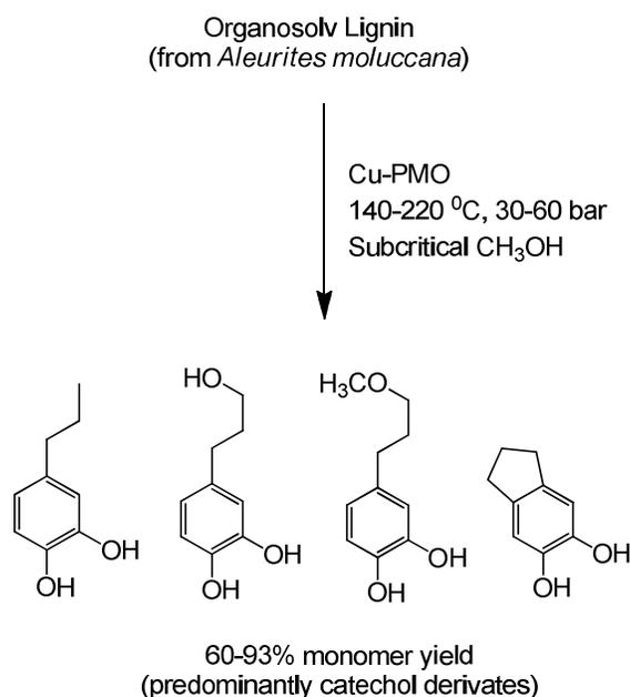
Scheme 14. Depolymerisation strategy involving the use of porous metal oxides (PMO) in subcritical methanol to produce lignin monomers composed mainly of catechol derivatives.<sup>38</sup>
