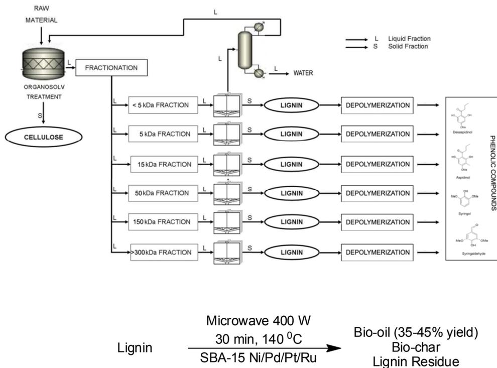
Scheme 11. Lignin purification and fractionation followed by heterogeneously catalyzed depolymerization using supported Ni nanomaterials to simple aromatics. Copyright Wiley-VCH Verlag GmbH & Co.KGaa. Reproduced with permission from reference 33b.
