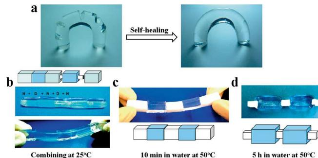
Fig. 9 Polymer-nanocomposite interaction-based PDMAAm and PNIPAAm self-healing hydrogels. (a) Self-healing of D-NC hydrogel with several knife cuts; (b) Self-healing of combined N-NC and D-NC hydrogels at 25°C for 48 h; (c) Changes of combined N-NC/D-NC hydrogels by immersing in 50°C water for 10 min and (d) 5 h, the N-NC sections are opaque and shrinking yet the D-NC sections are swelling. (Reprinted with permission from ref. 85. Copyright 2011, Wiley-VCH.)
