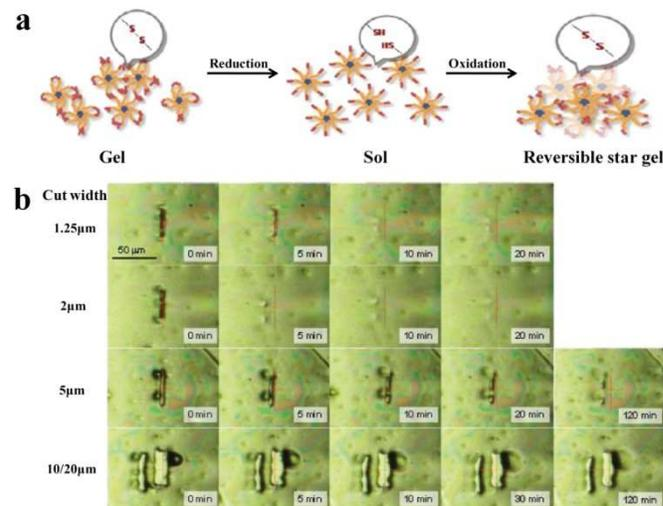
Fig. 12 Disulfide bond-based thiol/disulfide redox self-healing organogels. (a) Schematic illustration of the reversible gel film oxidized from the reductive SH-functionalized star polymers; (b) The optical microscope images of the self-healing process with initial cut width of 1.25, 2, 5, 10 and 20 μm, respectively. (Reprinted with permission from ref. 65. Copyright 2011, American Chemical Society.)
