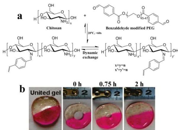
Fig. 13 Imine bond-based self-healing hydrogels. (a) chitosan-PEG hydrogel prepared by cross-linking of chitosan with benzaldehyde modified telechelic PEG; (b) The appearance of self-healing process between two different color semicircle hydrogels (the red one is stained by rhodamine B) and the hole punched in the middle of the united gel. (Reprinted with permission from ref. 64. Copyright 2011, American Chemical Society.)
