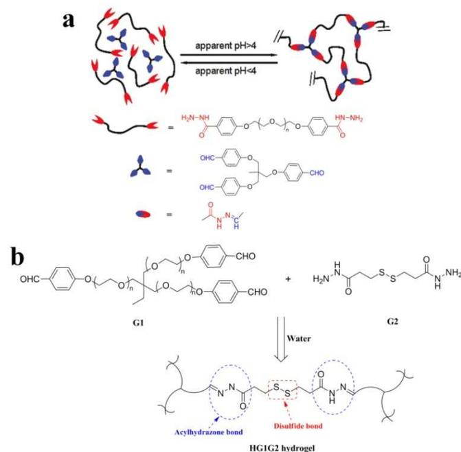
Fig. 14 Acylhydrazone bond-based self-healing gels. (a) The reversible polymer networks cross-linked by acylhydrazone bonds through condensation of acylhydrazines at the two ends of PEO with aldehyde groups; (Reprinted with permission from ref. 63. Copyright 2010, American Chemical Society.) (b) HG1G2 hydrogel contains both acylhydrazone and disulfide bonds. (Reprinted with permission from ref. 125. Copyright 2012, American Chemical Society.)
