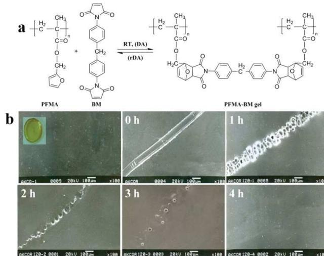
Fig. 16 DA reaction-based PFMA-BM organogel film. (a) Preparation of thermally reversible PFMA-BM gel through DA reaction; (b) SEM images of the PFMA-BM gel with a knife-cut healed for 1, 2, 3, and 4 h at 120°C, respectively. (Reprinted with permission from ref. 133. Copyright 2009, American Chemical Society.)
