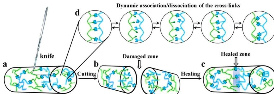
Fig. 1 Schematic illustration of self-healing mechanisms of self-healing gels based on CDC. (a) A cylindrical self-healing gel is cut by a knife; (b) The gel is cut into two pieces and the functional groups stay dissociated across the damaged zone; (c) The crack is healed by the reformed dynamic bonds after the fractured surface contacting each other; (d) The dynamic association and dissociation of the reversible cross-links based on CDC.
