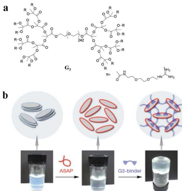
Fig. 8 Polymer-nanocomposite interaction-based dendritic self-healing hydrogel. (a) Schematic structures of dendritic macromolecules ( $G_3$ -binder); (b) The illustration and optical images for the fabrication procedures of SDM hydrogel. (Reprinted with permission from ref. 84. Copyright 2010, Nature publishing group.)
