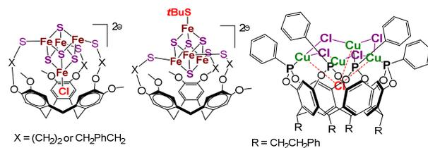
**Fig. 3** Left: [Fe<sub>4</sub>S<sub>4</sub>] cluster stabilized by a CTV ligand. Right: [Cu<sub>4</sub>Cl<sub>4</sub>] cluster stabilized by a calixarene ligand.
