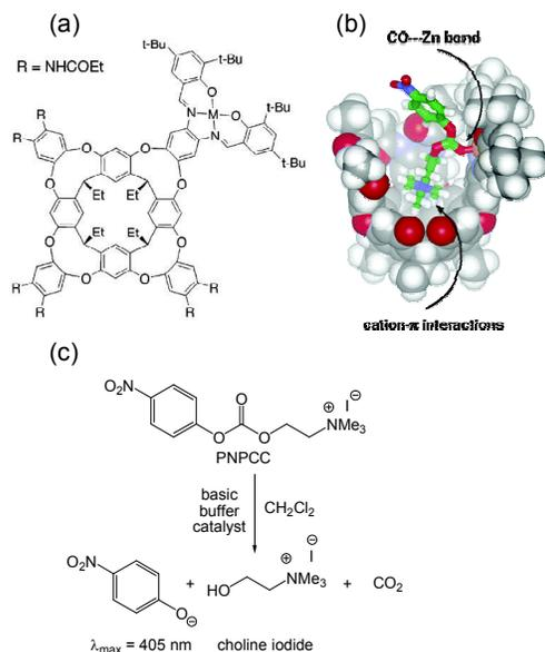
**Fig. 32** Hydrolysis of *p*-nitrophenylcholine carbonate by a  $\text{Zn}(\text{salen})$  complex grafted onto a deep cavitaand scaffold. The ammonium group of the substrate is recognized by the resorcinarene cavity (model in the center is reprinted with permission from Reference 74. Copyright 2004 American Chemical Society).
