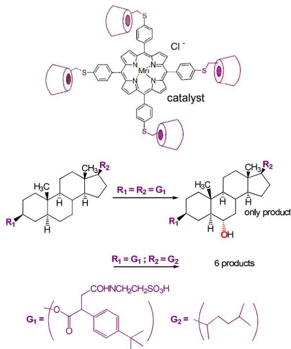
**Fig. 39** Breslow's cyclodextrin-appended Mn-porphyrin catalyst. Strong binding of the substrate in the CD receptors yields a single product obtained regio- and stereoselectively. Weak anchoring leads to a mixture of products.
