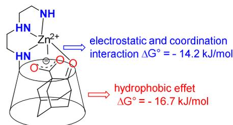
**Fig. 10** Early example of a  $\beta$ -CD  $\text{Zn}^{\text{II}}$  complex associating the hydrophobic effect for guest inclusion and the interaction of the ligand with a metal center.
