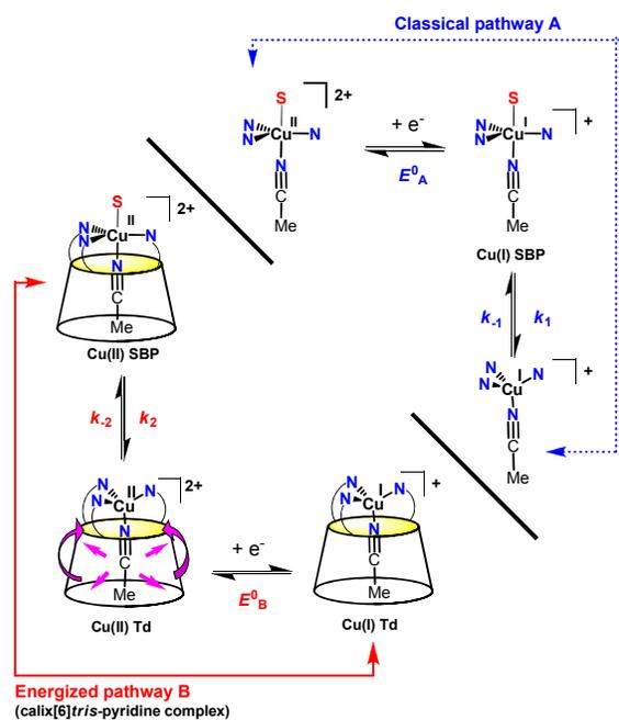
**Fig. 27** The two possible electron-transfer pathways for copper complexes associated with a SBP geometry at Cu<sup>II</sup> and Td geometry at Cu<sup>I</sup>. The structure of the calixarene is displayed in Fig. 16.
