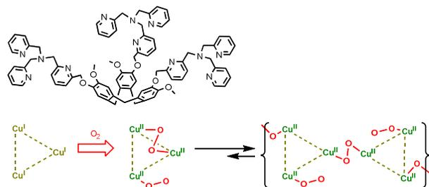
**Fig. 30** Trinuclear  $\text{Cu}^{\text{I}}$  complex derived from a Tris-TMPA-CTV scaffold. Interaction with  $\text{O}_2$  generates both a mononuclear  $\text{Cu}^{\text{II}}\text{-superoxo}$  and dinuclear trans-peroxo species.
