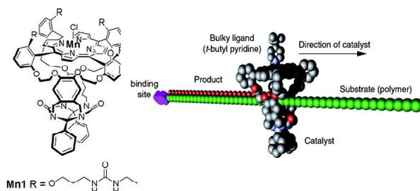
**Fig. 38** Structure of Nolte's processing oxidation catalyst. The polymer substrate threads through the catalyst ring and is oxidized within the cavity (model on the right is reprinted with permission from Reference 83. Copyright 2010 American Chemical Society).
