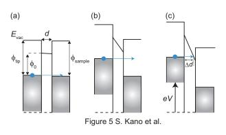
**Fig. 5** Schematic energy band diagram of three types of tunneling behaviors in metal/insulator/metal structures: (a)  $eV \simeq 0$ , (b)  $eV < \overline{\phi}$  and (c)  $eV > \overline{\phi}$ .  $\phi_0$  is a barrier height of the insulator,  $\overline{\phi}$  is an average barrier height of the insulator.  $\Delta d$  is a tunneling distance of an electron, and *d* is a thickness of the insulator.
