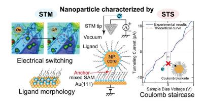
Scanning tunneling microscopy (STM) and scanning tunneling spectroscopy (STS) can characterize intriguing nanoparticle properties towards solid-state nanodevices.
