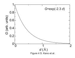
**Fig. 4** Typical relationship between transconductance (*G*) and thickness of materials (*d*) in vacuum.
