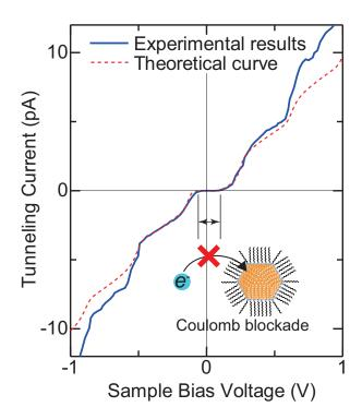
**Fig. 6** Typical experimental I - V characteristic of the DBTJ consisting of STM tip/vacuum/octanethiol ligand/Au core/decanedithiol anchor molecule/Au(111) substrate (solid line). Experimental Coulomb staircase is clearly observed. The dashed line represents the theoretical curve calculated by the orthodox theory. Inset is the schematic of Coulomb blockade effect that is observed near by V=0.
