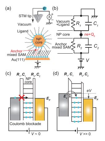
**Fig. 7** (a) Schematic image of DBTJs consisting of a single octanethiol protected Au nanoparticle on Au(111) surface. (b) Equivalent circuits of the DBTJs. (c)–(d) Schematic energy band diagrams of DBTJs. (c) Coulomb blockade condition. Electron tunneling is prohibited. (d) Allowed tunneling condition because of sufficient energy  $(E_c^+)$  given by voltage.
