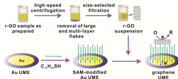
Fig. 6 Schematic illustration of r-GO nanoelectrode fabrication. Reprinted with permission from Ref. 61, copyright 2013, American Chemical Society.
