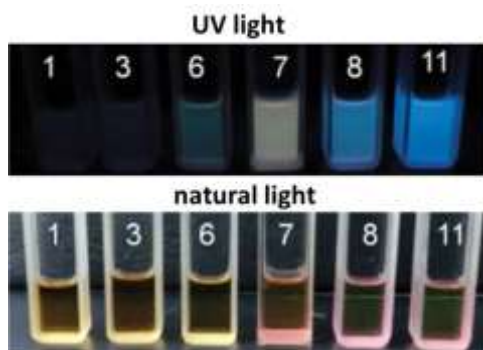
Fig. 13 Images of 313 in ethanol at different pH values under (A) a UV lamp and (B) natural light. The pH values are indicated on each vessel. Adapted with permission from Ref. 152. Copyright 2013 The Royal Society of Chemistry.
