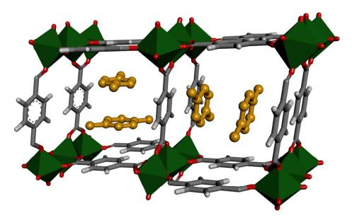
Figure 6. Pairwise stacking of pX (orange) in MIL-47(V) as determined by Rietveld refinement. (V: green; O: red; C: gray; H: white).
