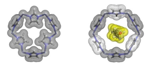
Figure 23. Flipping of the imidazolate groups of the "closed" window in ZIF-8 (left) allows for 1-butanol to enter through the now open window (right) and to be adsorbed in the cages.
