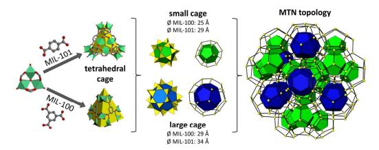
Figure 4. MTN topology of MIL-100( $M^{3+}$ ) and MIL-101( $M^{3+}$ ). Both frameworks are built up of  $M_3(\mu_3-O)(COO)_6(guest)_3$  trimeric SBUs forming tetrahedral cages by interconnection with six BDC linkers (MIL-101) or four BTC linkers (MIL-100) (left). These tetrahedral cages enclose two other types of cages, one featuring only pentagonal windows ("small cage") and the
