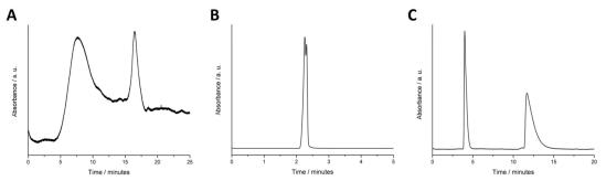
Figure 16. Separation of a mixture of ethylbenzene and styrene on a pure HKUST-1 column (A). Separation of the same mixture on an unmodified silica column (B). Separation of the same mixture on a silica column modified with HKUST-1 (C).<sup>92</sup>
