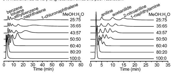
Figure 15. Effect of the mobile phase composition on the HPLC separation on a MIL-100(Fe) packed column (5 cm long x 4.6 mm i.d.): (left) benzene, toluene, ethylbenzene, naphthalene and 1-chloronaphthalene (5  $\mu$ L, 0.01 mol L<sup>-1</sup> each); (right) aniline, acetanilide, 2-nitroaniline and 1-naphthylamine (5  $\mu$ L, 0.01 mol L<sup>-1</sup> each).<sup>73</sup>
