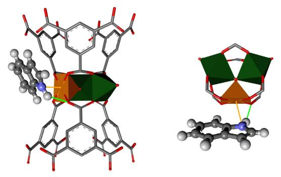
Figure 5. Adsorption of indole on MIL-100(V): Indole coordinates via the lone pair at N (blue) to the open V site (orange) and via hydrogen bonding (green) to the basic carboxylate moiety. (V: green/orange; O: red; C: gray; H: white)
