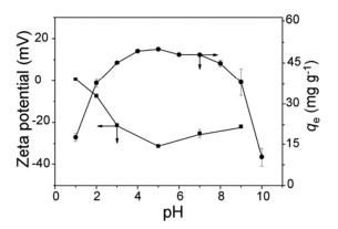
Figure 21. The  $\zeta$ -potential of MIL-100(Fe) (left vertical axis) and the amount of malachite green adsorption (right vertical axis) in function of pH. <sup>104</sup>
