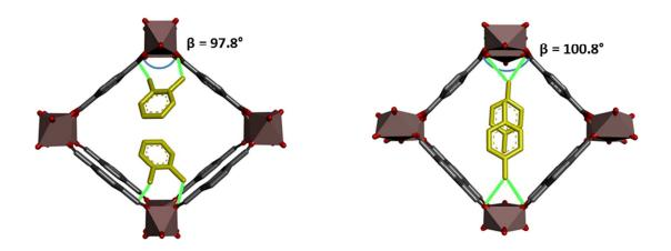
Figure 7. Adsorption of oX (left) and pX (right) in MIL-53(Al) as determined by Rietveld refinements. oX interacts with the framework through both methyl groups (green), while pX only interacts with one methyl group. This causes a stronger reduction of  $\beta$  in the case of oX.
