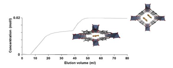
Figure 22. Breakthrough adsorption of phenol (0.02 M in water) over a 5 g MIL-53(Cr) column. The stepwise profile is attributed to the opening of the framework upon adsorption of phenol, allowing for additional phenol molecules (orange) to be stacked in the channels.<sup>105</sup>
