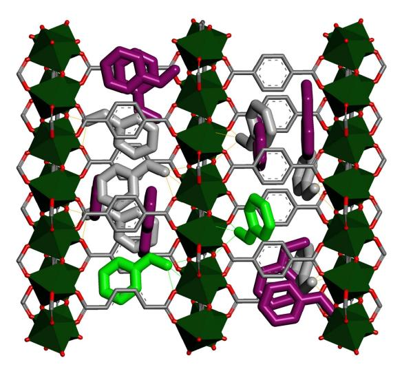
Figure 17. Stacking of ethylbenzene in styrene-loaded MIL-47. Styrene (purple) is packed pairwise in the channels of MIL-47, occupying several adsorption sites of ethylbenzene (gray). Only two of the possible adsorption sites for ethylbenzene are occupied (green).<sup>94</sup>
