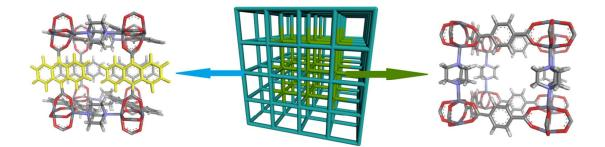
Figure 11. Core-shell functionalized particles of Zn<sub>2</sub>(BDC)(DABCO). The outer shell (blue) is functionalized with 9,10-anthracenedicarboxylate linkers (yellow), while the core (green) consists of BDC linkers. (Zn: dark blue; O: red; N: blue; C: gray; H: white)
