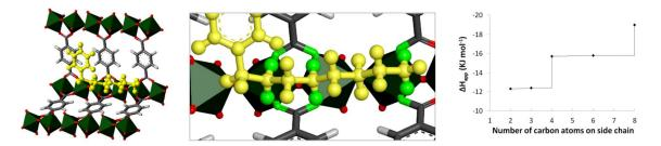
Figure 10. Adsorption of alkylaromatics in MIL-47. The apparent adsorption enthalpy increases stepwise with the length of the alkyl chain due to an increasing number of
