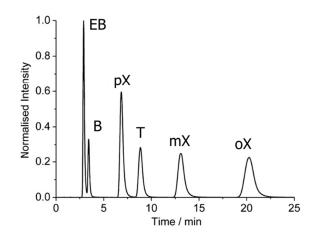
Figure 8. Pulse chromatogram of BTEX on a MIL-53(Fe) column at 323K with the order of elution: ethylbenzene (EB), benzene (B), *para*-xylene (pX), toluene (T), *meta*-xylene (mX) and *ortho*-xylene (oX).<sup>59</sup>
