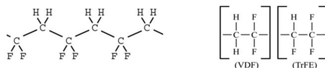
Figure 1: Sketch of the PVDF polymer chain and of the VDF and TrFE monomers. The large difference in electronegativity between the Hydrogen and Fluorine atom, along with an all-trans configuration and parallel stacking of the polymer chains are responsible for the large spontaneous polarization possible in VDF and its copolymers. TrFE is added to reduce the size of the VDF crystallites and allows for electrical poling at lower, more manageable fields.
