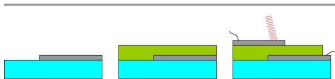
Figure 2: The sample is prepared by thermal evaporation of aluminium onto a clean glass substrate, followed by spincoating the thin polymer film and capping it with another thermally vapour-deposited aluminium electrode. The top electrode functions as absorbing material for the modulated laser beam and both electrodes are used to measure the induced surface charges and to apply the external poling field.
