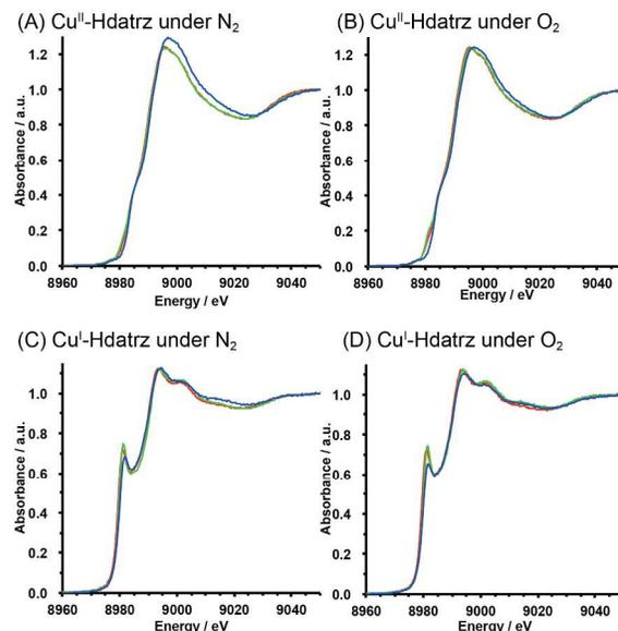
**Fig. 4** *In situ* XANES spectra of Cu/KB in the oxidation state of Cu<sup>II</sup> (A) under N<sub>2</sub> and (B) under O<sub>2</sub>, and in the oxidation state of Cu<sup>I</sup> (C) under N<sub>2</sub> and (D) under O<sub>2</sub>. The red, green and blue traces indicate the spectra recorded at pH 7, pH 10 and pH 13, respectively. Bias potentials applied are as follows: +0.95 V
