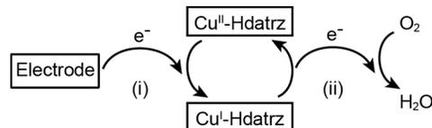
**Scheme 2** Simplified electron transfer steps in the Cu-Hdatrz/KB system: (i) electron transfer from the electrode/KB to Cu<sup>II</sup>-Hdatrz and (ii) electron transfer from Cu<sup>I</sup>-Hdatrz to O<sub>2</sub> (the ORR step).
