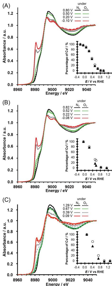
**Fig. 3** *In situ* fluorescent XANES spectra of Cu/KB (A) at pH 7, (B) at pH 10 and (C) pH 13. The solid line and dashed lines indicate the XANES spectra that were recorded under nitrogen and oxygen, respectively. Insets: plots of percentages of Cu<sup>I</sup> vs applied potential (open circle: under nitrogen; filled triangle: under oxygen). The percentages were calculated based on the results of the linear combination analysis of the XANES spectra of Cu/KB and fully reduced Cu/KB.
