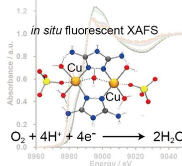
*In situ* XAFS studies on a copper catalyst revealed that deprotonation from the triazole ligand might cause the coordination geometrical changes, resulting in enhancement of the oxygen reduction reaction activity.
