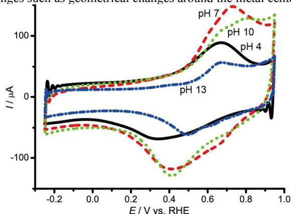
**Fig. 1** CVs of Cu/KB in Britton-Robinson buffered aqueous solutions (0.04 M) containing 0.1 M NaClO<sub>4</sub> at pH 4 (solid line in black), 7 (dashed line in red), 10 (dotted line in green) and pH 13 (alternate long and short dashed line in blue). All CVs shown here were recorded at a sweep rate of 100 mV s<sup>-1</sup> under Ar.
