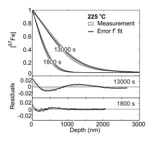
**Fig. 4** The tail of each diffusion profile was fit with an error function solution (Eq. 4. Example fits for two samples annealed at 225 °C for approx. 1800 and 13000 s are shown.
