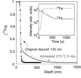
**Fig. 3** The interdiffusion of a 130 nm-thick  ${}^{57}$ Fe deposit on Fe<sub>1-x</sub>S crystals was measured by secondary ion mass spectrometry (SIMS). The black curve shows the SIMS profile from an unannealed sample, indicating the depth of the original deposit. Inset: raw SIMS data for a sample annealed for 5 minutes at 275 °C; converted in the main plot to  ${}^{57}$ Fe concentration vs. depth into the crystal (grey curve).
