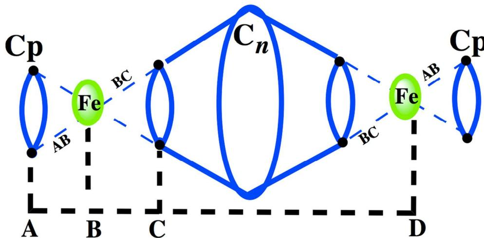
**Scheme 2** Schematic representation of buckyferrocene systems where Cp is cyclopentadiene ring and  $C_n$  represents  $C_{30}$ ,  $C_{60}$  and  $C_{70}$  fullerenes and their fragments
