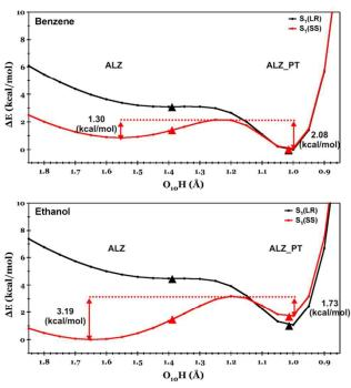
**Figure 2.** Potential  $S_1$  energy curves as a function of the  $O_{10}H$  distance computed in benzene (top) and ethanol (bottom). The red and black lines are obtained using the LR and SS approaches, respectively.  $\blacktriangle$  and  $\bigstar$  markers indicate the LR and the SS stabilities computed on the freely
