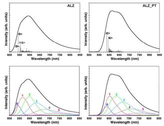
**Figure 4.** Emission spectra computed in benzene of ALZ (left) and ALZ\_PT (right) with the main vibronic transitions involved (top) and decomposition of the spectra in contributions from the 0-0 transition (0) and the n (n=1,5) simultaneously excited oscillators (bottom).
