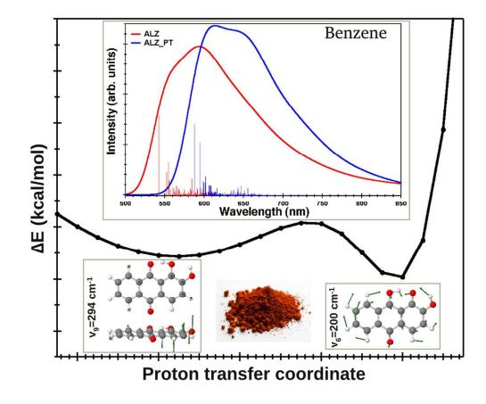
Potential energy curve for the ESIPT. Top Inset: Vibrationally resolved emission computed for both tautomers. Bottom inset: main vibrational modes.
