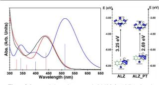
Figure 3 Computed absorption spectra in DMSO for ALZ (red) and ALZ\_PT (blue) compared to the experimental absorption spectrum of alizarin in a mixture of DMSO:water (50:50).[42] Right: ALZ and ALZ\_PT frontier molecular orbitals energies and isodensiy plots computed in DMSO
