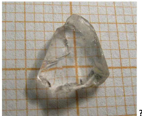
Fig. 1. Single crystal \text{MgSrF}_4 sample, 2 mm thick.
