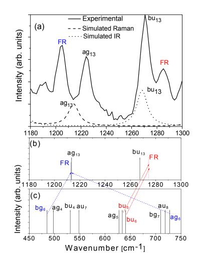
Figure 12. (a) The experimentally Fermi resonance and simulated TER spectra of DMAB for Raman-active ag13 and IR-active bu13 modes. (b) and (c) The calculated vibrational modes and the combinational modes for Fermi resonance. Figure 12 is taken from Ref. [45].
