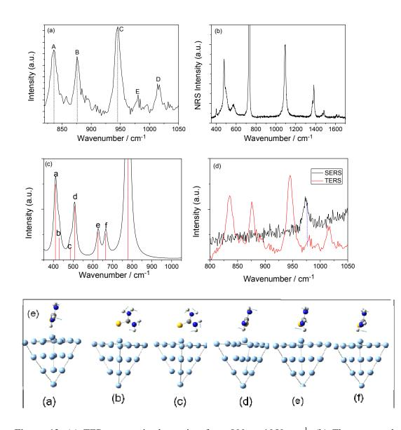
**Figure 13.** (a) TER spectra in the region from 800 to 1050 cm<sup>-1</sup>. (b) The measured Raman spectra of the thiourea powder (c) The calculated Raman spectra of thiourea adsorbed on the  $Ag_{20}$  cluster in the thione form (d) The measured TER and SERS spectra from 800 to 1050 cm<sup>-1</sup> (e) The calculated vibrational modes. Figure 13 is taken from Ref. [46].
