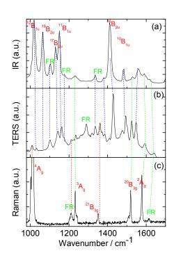
**Figure 8.** Vibrational spectra of pyrazine. (a) The measured IR vibrational spectrum of pyrzaine powder. (b) The HV-TER spectra of pyrazine adsorbed on Ag the film. (c) The Raman spectrum of pyrzaine powder. Figure8 is taken from Ref. [4].
