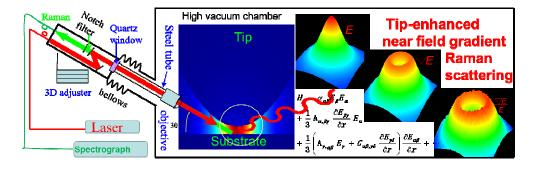
**Fig 1.** The scheme of HV-TERS setup, and the near field gradient effects on HV-TERS, which is taken from Ref. [4].
