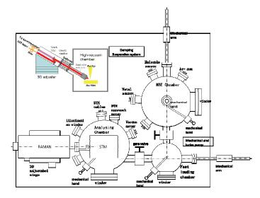
**Figure 2.** Scheme of the HV-TERS system with a preparing MBE chamber, a fast loading chamber and a TERS Analysis chamber.
