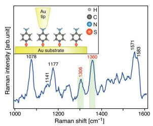
**Figure 11.** TER spectrum of DMAB produced from PATP molecules sandwiched between Au substrate and Au tip, as illustrated in the inset. Figure 11 is taken from Ref. [33].
