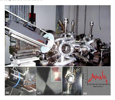
**Figure 3.** (a) Picture of the actual finished HV-TERS system. (b) The core part of TERSobjective and STM tip. (c) Image of the tip and the reflected tip by the substrate. The inset is when tip was illuminated with a 633nm laser. (d) the  $Ar^+$  gun cleaning and MBE part in the MBE chamber. (e) The atomic resolved image of graphite (7×7nm<sup>2</sup>). The inset is a Raman spectrum from a sample with PATP molecules on Au surface.
