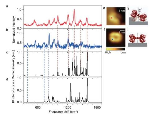
Figure 14 (a) and (b) Single-molecule TERS spectra for an isolated  $H_2$ TBPP molecule adsorbed on the terrace or at the step edge. (c) and (d) Calculated TERS spectra of  $H_2$ TBPP. (e) and (g) STM image and schematic image of  $H_2$ TBPP molecule flatly adsorbed on Ag substrate. (f) and (h) STM image and schematic image of tilted  $H_2$ TBPP molecule with tilt angle of 30°. Figure 14 is taken from Ref. [8].
