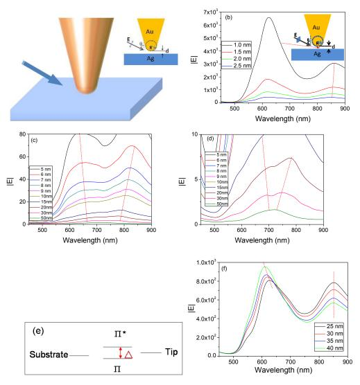
**Figure 4.** (a) The theoretical model for the TERS. (b)-(d) The distance dependent SPRs, (e)SPR hybridization model of TERS. (f) Tip radius dependent plasmonic peaks. Figure 4 is taken from Ref. [46].
