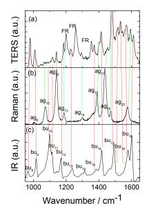
**Figure 9.** (a) The TER spectrum of DMAB adsorbed on the gold film. (b) Raman spectrum of DMAB powder. (c) The IR vibrational spectrum of DMAB. Figure 9 is taken from Ref. [10].
