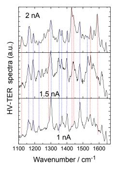
**Figure 7.** The tunneling current intensity dependent TER spectra of 2,2'DA-DMAB produced from 2,4-DNBT. Figure 7 is taken from Ref. [3].
