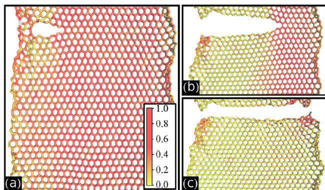
**Fig. 7** (Color online) Typical snapshots from MD simulations showing different stages of the mechanical failure of an armchair silicene membrane under mechanical strain. The scale goes from low stress (yellow/lighter) to high stress (red/darker).
