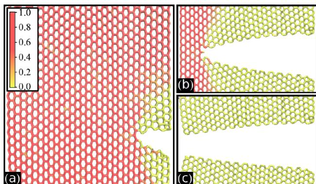
**Fig. 6** (Color online) Typical snapshots from MD simulations showing different stages of the mechanical failure of a zigzag silicene membrane under mechanical strain. The scale goes from low stress (yellow/lighter) to high stress (red/darker).
