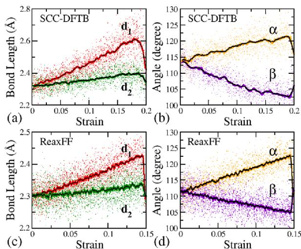
**Fig. 3** (Color online) Bonds length and angles values for ACM.  $d_1$  is represented by green line,  $d_2$  is represented by red line,  $\alpha$  orange line and  $\beta$  is represented by violet line.
