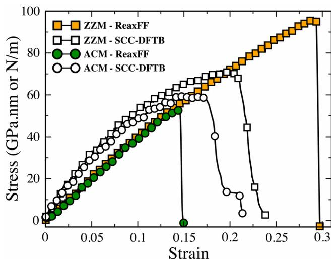
**Fig. 2** (Color online) Stress versus strain curves for zigzag and armchair edge terminated structures. Results for the temperature of 150K and for both ReaxFF and SCC-DFTB methods. See text for discussions.
