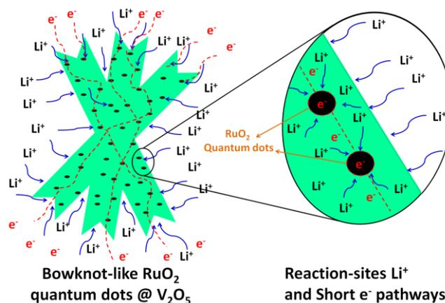
Scheme 1. Schematic illustration of the bowknot-like RuO<sub>2</sub> quantum dots @ V<sub>2</sub>O<sub>5</sub> with accessible intercalation sites for Li<sup>+</sup> and short electron/ion transport pathways.
