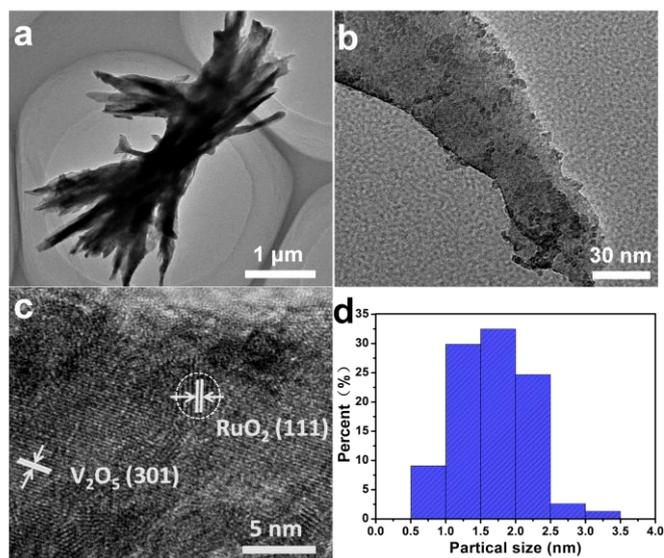
**Figure 2** (a) The low, (b) the high magnification TEM images and (c) the high-resolution TEM (HRTEM) images of the annealed RQDV, respectively. (d) Particle size distribution of RuO<sub>2</sub> QDs on V<sub>2</sub>O<sub>5</sub>.
