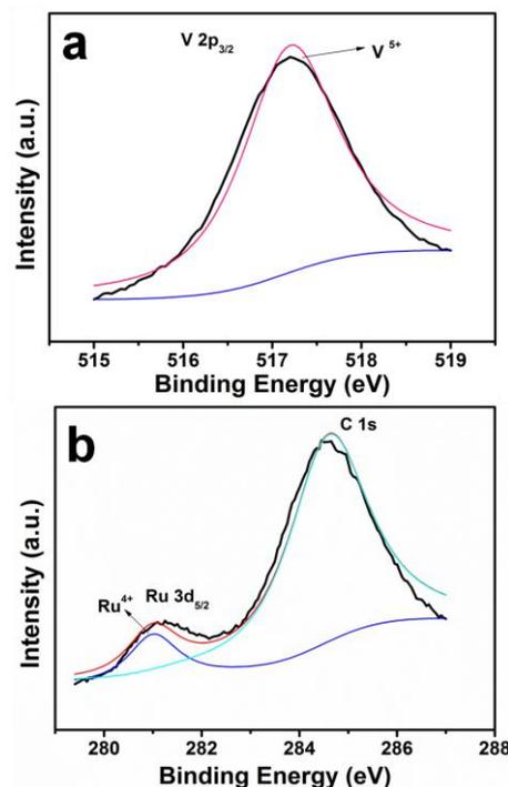
**Figure 3** The XPS spectra for annealed RQDV: (a) the V 2p<sub>3/2</sub> bands; (b) the Ru 3d<sub>5/2</sub> and C1s bands.
