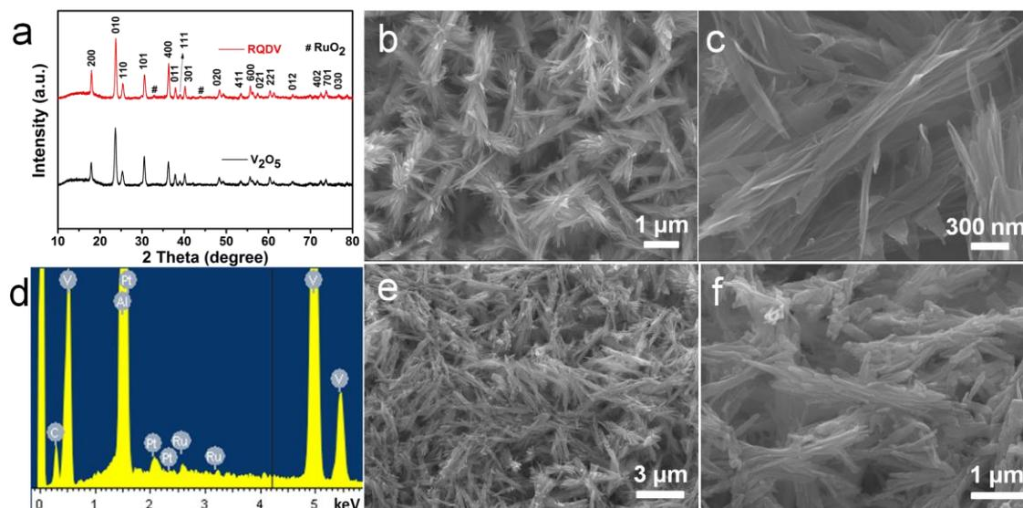
Figure 1 (a) The XRD patterns of the prepared  $V_2O_5$  and RQDV; (b-c) the low and high magnification FESEM images of RQDV precursor, respectively; (d) The EDX pattern of RQDV; (e-f) the low and high magnification FESEM images of RQDV, respectively.
