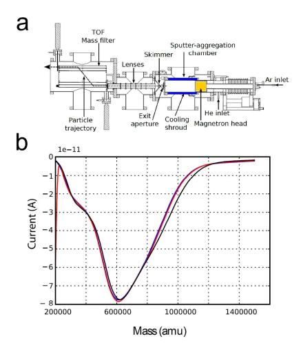
**Figure 5:** a) Scheme of the Birmingham cluster source used to deposit size selected nanoparticles. b) Current versus mass deposition curves taken keeping the pressure in the sputter-aggregation chamber constant. The three deposition curves were collected at time intervals of 15 minutes.
