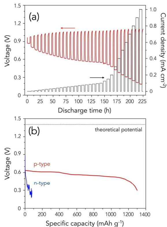
**Fig. 4** (a) Dynamic step discharge response of the p-type Ge-air cell (p+++), when operated at increasing current drains. (b) Long-term discharge profiles of n-type Ge and p-type Ge anodes (both heavily doped), showing the huge difference in the electrochemical performance in a Ge-air cell using a 6.0 M gelled KOH electrolyte at a discharge current of 50  $\mu\text{A cm}^{-2}$ .
