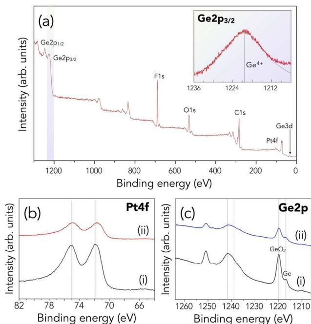
**Fig. 5** X-ray photoelectron spectra of the cathode and anode after full discharge for 700 hr. (a) XPS survey scan of the Pt/C cathode after discharge, while the inset shows the X-ray photoelectron spectrum of Ge $2p_{3/2}$ , fitted with the Ge $^{4+}$  spectrum. (b) Pt $4f$  XP spectra of Pt/C cathode (i) before and (ii) after full
