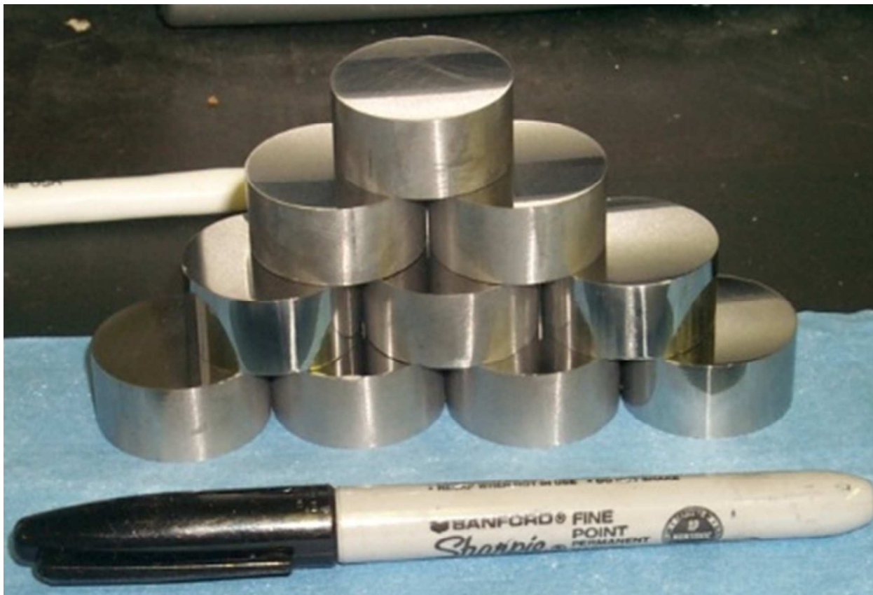
Figure 2. Ten 80 g ingots of p-type skutterudite as sintered by GM R&D. These pucks are diced into wafers and processed into TE elements.
