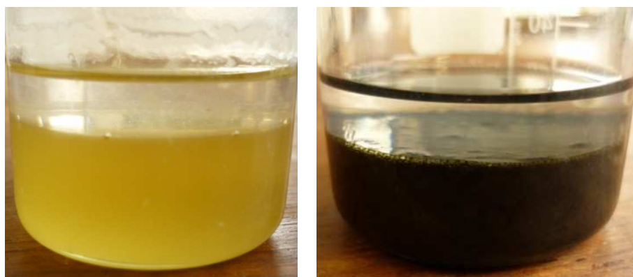
Fig. 2: Photographs of phase behaviour of decane with a) [AlCl_2, urea]^+ AlCl_4^- b) as (a) with 20 vol % toluene.
