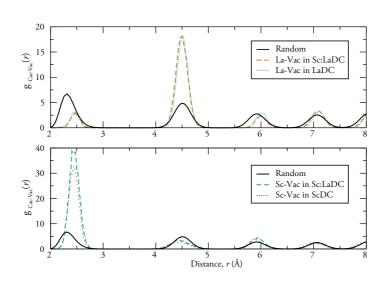
**Fig. 8** Cation–vacancy partial radial distribution functions ( $g_{Cat-Vac}(r)$ ) at 873 K. Top panel: Random (solid black line),  $La^{3+}$  – Vacancy in Sc:LaDC (dashed orange line) and  $La^{3+}$  – Vac in LaDC (dotted turquoise line). Bottom panel: Random (solid black line),  $Sc^{3+}$  – Vacancy in Sc:LaDC (dashed green line) and  $Sc^{3+}$  – Vacancy in ScDC (dotted magenta line)
