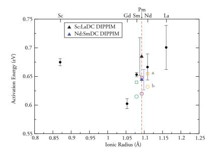
**Fig. 7** DIPPIM activation energies (eV) for  $Ce_{0.90}RE_{0.10}O_{1.95}$  from Figure 4 along with those for the co-doped systems, Nd:SmDC (filled blue triangle) and Sc:LaDC (filled black triangle). Experimental values from a) Omar *et al.*<sup>37</sup> (open squares) and b) Kasse and Nino<sup>46</sup> (open circles) with green for SmDC, maroon for Nd:SmDC and orange for NdDC.
