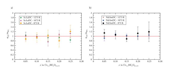
Fig. 6 DIPPIM ionic conductivities shown as a ratio of the values for co-doped (CD) ceria divided the weighted average (WA) of their singly-doped parent oxides. Panel a) corresponds to the Sc:LaDC system and panel b) corresponds to Nd:SmDC.
