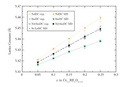
**Fig. 5** DIPPIM calculated (filled symbols) and experimental (open symbols) lattice constants from Buyukkilic *et al.*<sup>81</sup> at 300 K for for  $Ce_{1-x}RE_xO_{2-x/2}$ , where x = 0.05, 0.10, 0.15, 0.20, 0.25 and RE = Sm (diamonds), Nd (triangles pointing left), Nd:SmDC (squares) and Sc:LaDC (triangles pointing down). The lines shown are intended as a guide to the eye only.
