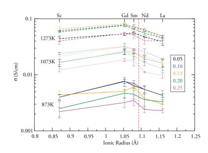
**Fig. 2** Ionic conductivities for singly doped ceria ( $Ce_{1-x}RE_xO_{2-x/2}$ ) at 1273 K (blue diamonds), 1073 K (black dots) and 873 K (red triangles). The vertical dashed red line represents the critical ionic radius ( $r_C$ ) introduced by Andersson *et al.*<sup>29</sup>.
