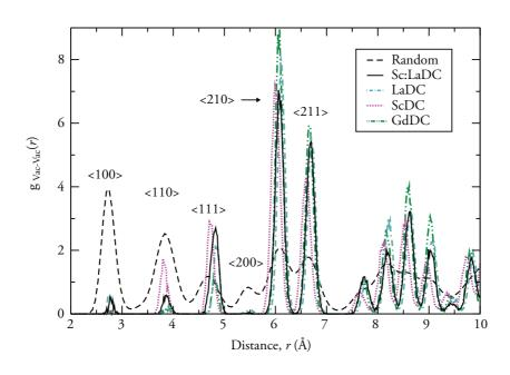
**Fig. 9** Vacancy–vacancy partial radial distribution functions at 873 K for Sc:LaDC (solid black line), LaDC (dot-dashed turquoise line), ScDC (dotted magenta line), GdDC (dot-dot-dashed green line) and a random vacancy distribution (O–O g(r)). The <100>, <110> and <111> labels indicate different directions along the simple cubic anion sublattice.
