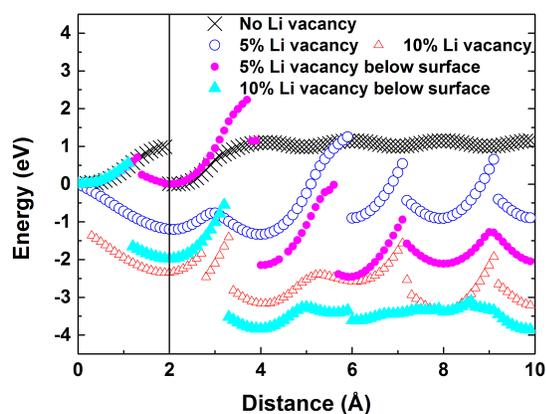
Figure 6. The effects of Li-deficiency on the Li surface diffusion barriers. Vertical solid line denotes the location of LiF surface at 2 Å, bulk LiF is at larger distances. Li adatom started at 0 Å.
