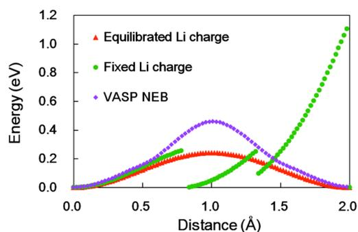
Figure 1. Li diffusion bulk in bulk LiF. Only the initial Li is moved here.
