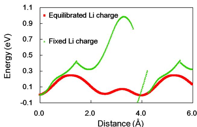
Figure 9.  $\text{Li}^+$  diffusion barrier along the Fe(111)/LiF(001) interface.
