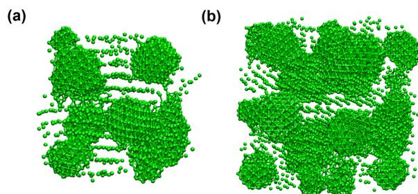
Figure 10. The interconnected Fe network after reaction of  $\text{FeF}_2$  to Li (LiF and remaining  $\text{FeF}_2$  not shown here) for (a) a  $3\text{nm} \times 3\text{nm} \times 3\text{nm}$  cluster and (b) a  $5\text{nm} \times 5\text{nm} \times 5\text{nm}$  cluster.
