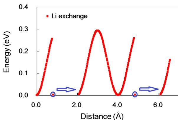
Figure 3.  $\text{Li}^+$  bulk diffusion barrier with exchange mechanism. Circles indicate the position of an exchange. Arrows show that during the exchange, the new diffusing  $\text{Li}^+$  has moved forward along the diffusion direction and after exchange its energy is monitored, thus leading to a sudden increase in the x-axis distance coordinates.
