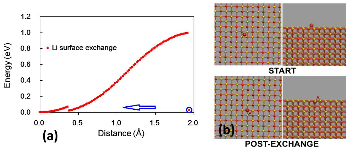
Figure 5. (a) Energy of  $\text{Li}^+$  surface exchange. Circles indicate the position of the exchange. Arrows show that after exchange, the new diffusion atom is pushed away from the surface. Surface locates at  $2.0\text{\AA}$ . (b) Top (left) and side (right) views of the inserting Li (large red) exchanging for the lattice Li (small red) in LiF crystal surface. Yellow are F ions.
