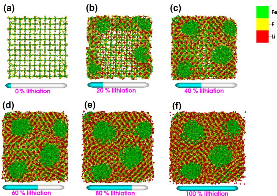
Figure 8. Structural evolution of an  $\text{FeF}_2$  nanoparticle exposed on all sides to Li ions during a conversion reaction (red=Li, yellow = F, green=Fe). Notice that only one surface is depicted, the pattern is similar on other surfaces.
