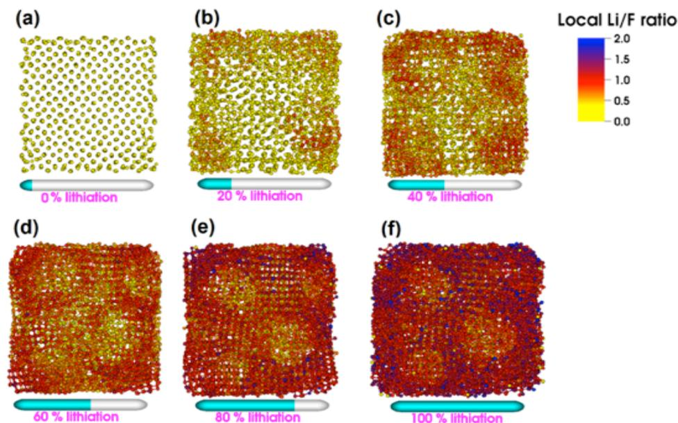
Figure 7. Evolution of the local Li concentration during a conversion reaction in an  $\text{FeF}_2$  nanoparticle. A ratio of 1.0 indicates the correct stoichiometry in a LiF crystal. Smaller ratio indicates Li deficiency and larger ratio indicates Li segregation. Empty regions are occupied by Fe clusters (not shown).
