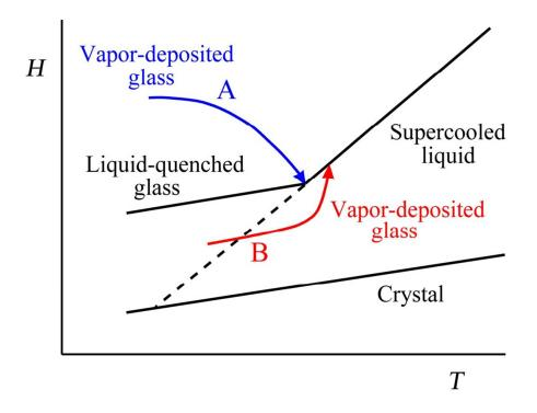
Fig. 1 Schematic presentation of the relations among the temperature dependences of *H* in different states of a molecular compound. See the text for the symbols A and B. Reproduced from Ref. 25 by permission of the Society of Rheology, Japan.
