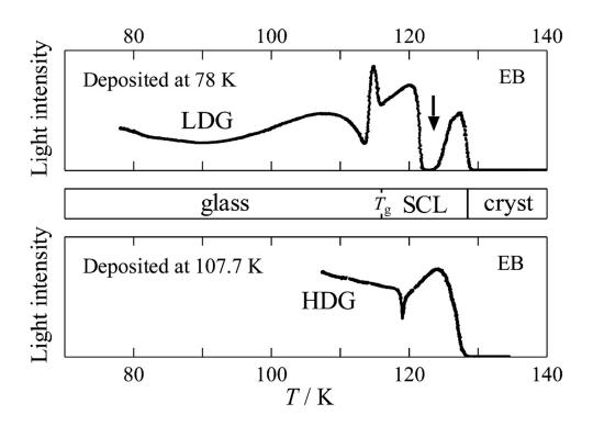
Fig. 9 Comparison of the evolution of the reflected-light intensity of two types of vapor-deposited EB samples, and the temperature regions distinguished with the sample states. Reproduced from Ref. 83 by permission of The Chemical Society of Japan.
