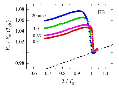
Fig. 11 Evolution of  $V_{\rm m}$  due to the temperature elevation of the EB samples deposited at 78 K with different  $v_{\rm d}$ . The vertical and the horizontal axes represent the  $V_{\rm m}$  and T normalized in the same manner as those in Fig. 6, respectively.
