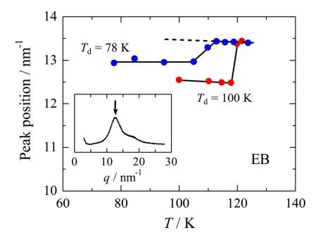
Fig. 14 Evolution of peak position of the broad diffraction pattern observed for TL glasses deposited at 78 K and 100 K with the stepwise temperature elevation. Insertion indicates the initial diffraction pattern of the sample deposited at 100 K. Arrow indicate the peak position.
