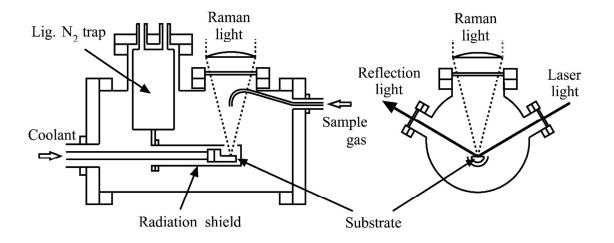
Fig. 4 Construction of a vacuum chamber for the Raman and reflected-light intensity measurements on vapor-deposited glasses.
