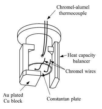
Fig. 5 DTA sensor with a light-reflecting mirror for in situ and simultaneous monitoring of thermal and optical behaviors of a vapor-deposited molecular films.
