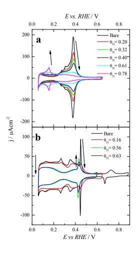
**Figure 1.** Evolution of the voltammetric profiles in 0.5 M H<sub>2</sub>SO<sub>4</sub> with increasing amounts of Tl on (a) Pt(100) and (b) Pt(111). Scan rate: 0.05 V s<sup>-1</sup>. Arrows indicate changes associated with increasing Tl amounts at the surface.
