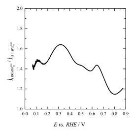
**Figure 6.** Ratio between the HCOOH oxidation current densities obtained with Tl-modified (maximum coverage) (100) and (111) Pt nanoparticles. Data taken from figure 4.
