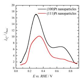
**Figure 5.** Ratio between the HCOOH oxidation current densities obtained with the bare and Tl-decorated (maximum coverage) shape-controlled Pt nanoparticles. Data taken from figure 4.
