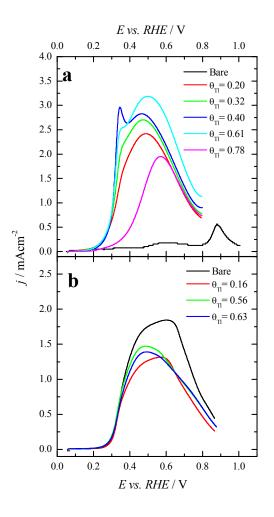
**Figure 2.** Positive sweep voltammetric profiles for 0.1 M formic acid oxidation in 0.5 M  $H_2SO_4$  with and without Tl for (a) Pt(100) and (b) Pt(111) single crystals. Scan rate:  $0.02 \text{ V s}^{-1}$ .
