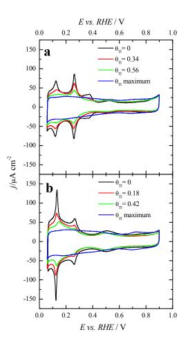
**Figure 3.** Voltammetric profiles for increasing amounts of Tl coverages on (a) (100)Pt and (b) (111)Pt nanoparticles in 0.5 M  $\rm H_2SO_4 + 10^{-4} \sim 10^{-5}$  M  $\rm Tl_2SO_4$ . Scan rate: 0.05  $\rm Vs^{-1}$ .
