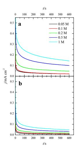
**Figure 10.** Current transients for (a) (100)Pt and (b) (111)Pt nanoparticles with maximum Tl coverage recorded at 0.20 V for different formic acid concentrations in 0.5 M H<sub>2</sub>SO<sub>4</sub>.
