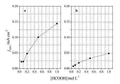
**Figure 11.** Comparison between formic acid concentrations and current densities obtained after 10 minutes at 0.2 V. Data extracted from Fig. 9 for (a) (100)Pt and (b) (111)Pt nanoparticles.
