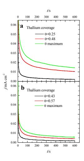
**Figure 7.** Current transients recorded at 0.2 V for formic acid electrooxidation for (a) (100)Pt and (b) (111)Pt nanoparticles with different Tl coverages. Test solution: 0.1 M formic acid in 0.5 M H<sub>2</sub>SO<sub>4</sub>.
