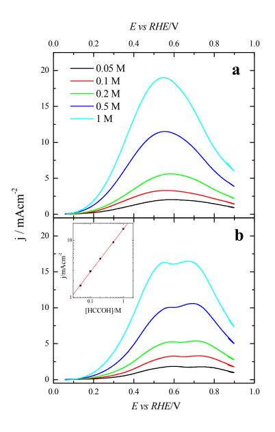
**Figure 9.** Positive sweep voltammetric profiles for (a) (100)Pt and (b) (111)Pt nanoparticles with maximum Tl coverage in different concentrations of formic acid in 0.5 M H<sub>2</sub>SO<sub>4</sub>. Scan rate: 0.02 Vs<sup>-1</sup>. Insert: double logarithmic plot of the current density at 0.5 V for the (111)Pt nanoparticles vs. formic acid concentration
