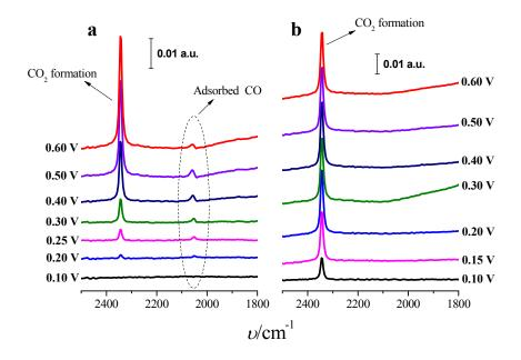
**Figure 8.** *In situ* FTIR spectra for formic acid electro-oxidation on (100)Pt nanoparticles: (a) bare Pt and (b) maximum Tl coverage. Reference spectra were taken at 0.05 V. Test solution: 0.05 M formic acid in 0.1 M H<sub>2</sub>SO<sub>4</sub>.
