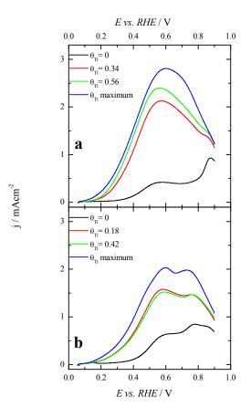
**Figure 4.** Positive sweep voltammetric profiles for formic acid electro-oxidation with increasing amounts of Tl coverages for (a) (100)Pt and (b) (111)Pt nanoparticles. Scan rate: 0.02 Vs<sup>-1</sup>. Test solution: 0.1 M formic acid in 0.5 M H<sub>2</sub>SO<sub>4</sub>.
