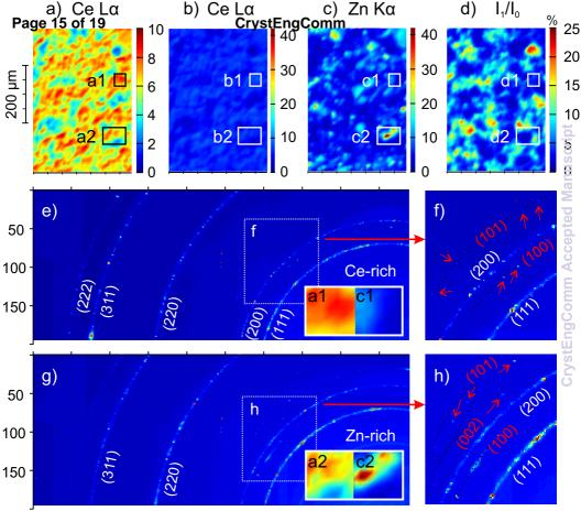
Seemingly monophasic Zn-doped ceria nanocrystals contain substantial amounts of x-ray amorphous ZnO not detectable by standard XRD. This ZnO can be incorporated upon annealing at temperatures up to  $1300\,^{\circ}$ C.
