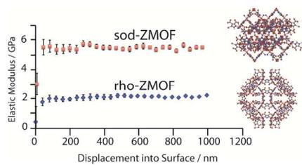
We report the low elastic modulus of a zeolitic MOF, along with stabilization against structural collapse by filling with solvent.
