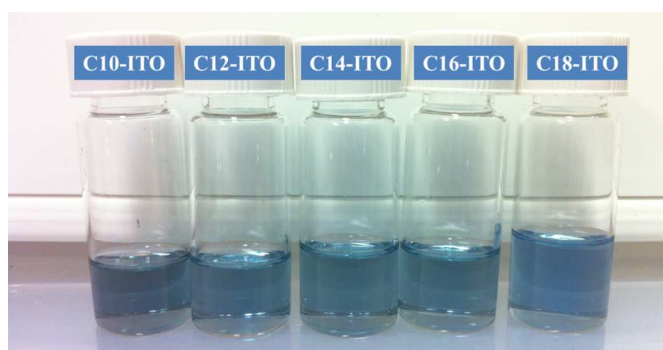
Fig. 6 A photo of ITO nanocrystal dispersions in chloroform. The concentration is 10 mg/mL.
