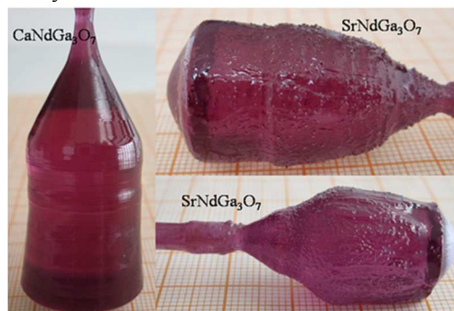
Fig. 1 The as-grown \text{CaNdGa}_3\text{O}_7 and \text{SrNdGa}_3\text{O}_7 single crystals pulled along [001] -direction.
