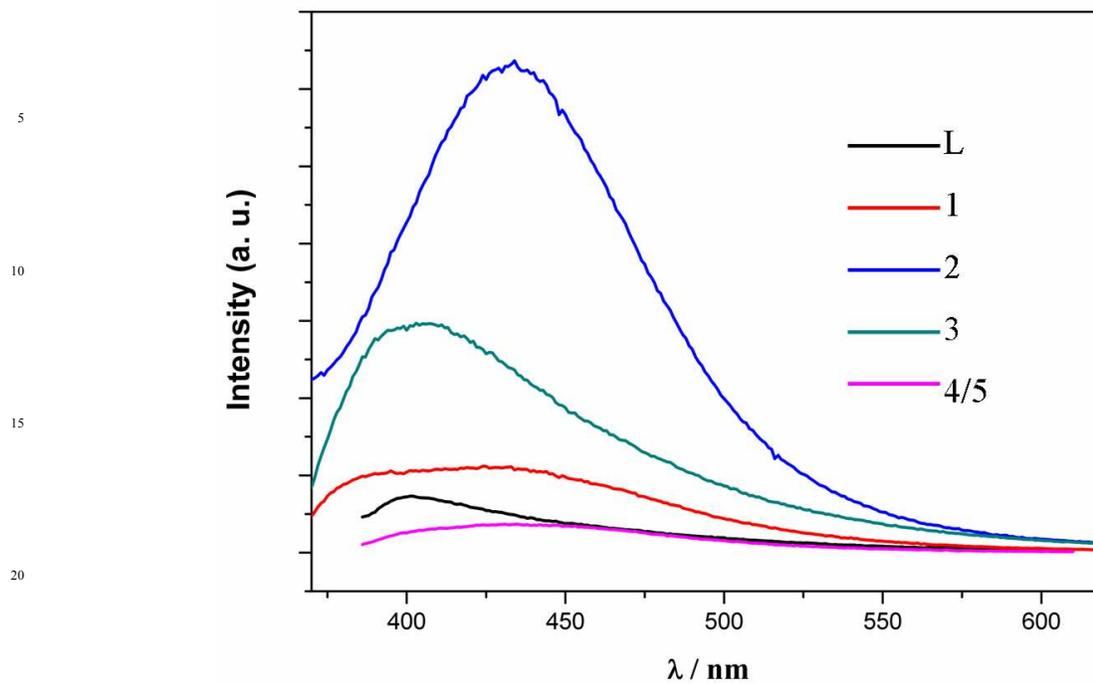
25 **Fig. 5.** The fluorescent spectra of 1-5 and L(H<sub>4</sub>dcppa) in the solid-state at room temperature.
