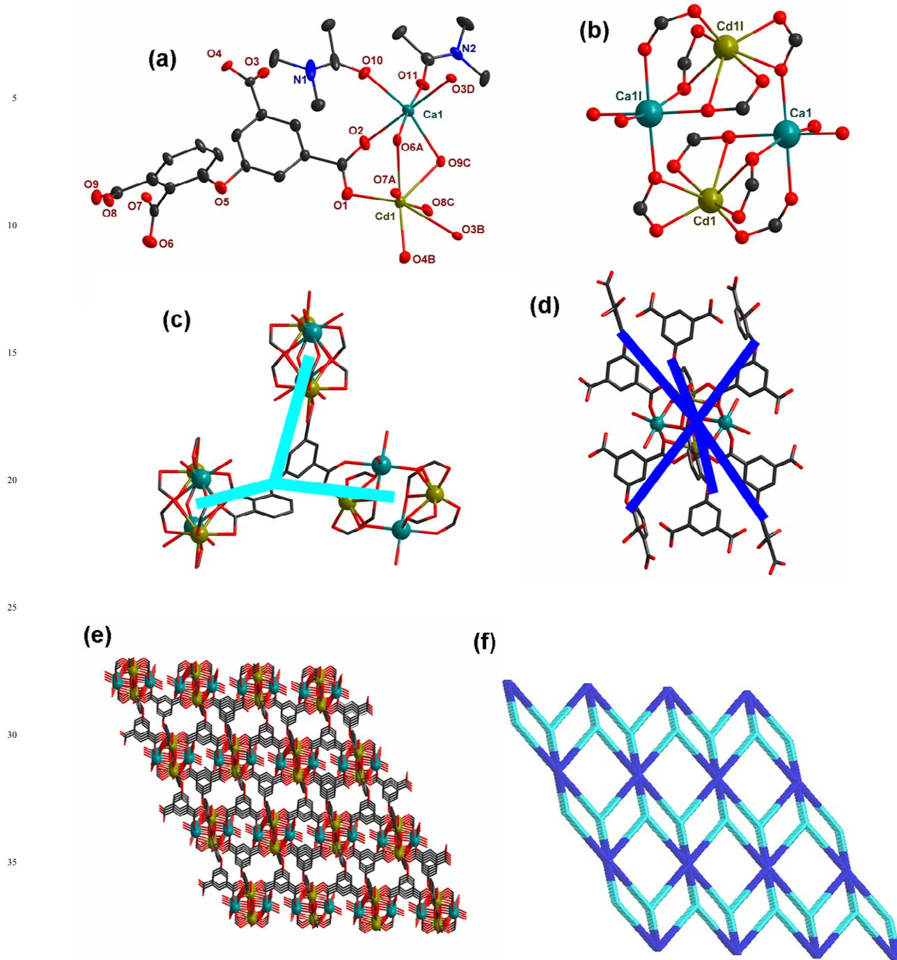
40 **Fig. 2.** View of **2**: (a) the coordination environments of Cd(II) and Ca(II) ions with 40% thermal ellipsoids. (b) the tetranuclear  $[\text{Cd}_2\text{Ca}_2(\text{COO})_8(\text{DMA})_4]$  building unit. (c) each  $(\text{dcpa})^{4-}$  ligand surrounded by three tetranuclear  $\text{Cd}_2\text{Ca}_2$  units to form a 3-
