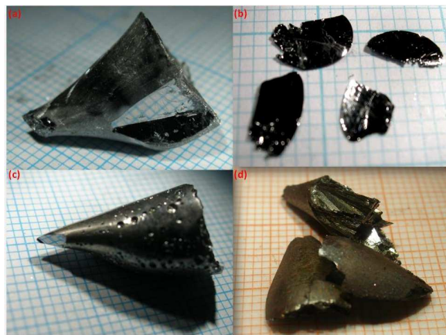
Fig.3 Single crystals grown from three different growth methods, (a) melt growth, (b) chemical vapor transport (CVT), and (c) Bridgman growth. Bridgman growth of Mn x BiTeI (x=0.1) is shown in (d) after it is stored in the air for one day. A thin brown film is coated on the surface to indicate that the sample is hygroscopic for Mn x BiTeI.
