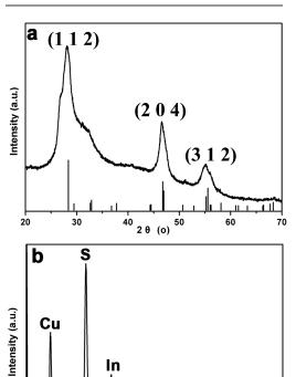
Figure 2. XRD pattern (a) and EDX spectrum (b) of the as-prepared CIS nanospheres. The vertical lines in (a) indicate the peak positions for the standard chalcopyrite phase CIS (JCPDF No. 85-1575).
