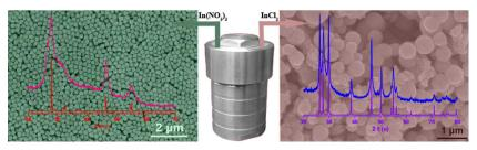
Monodisperse chalcopyrite and wurtzite  $CuInS_2$  nanocrystals are produced and their crystal phases are controlled by varying the In precursors.
