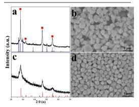
Figure 4. XRD patterns and SEM images of the as-prepared samples with different  $R_{\rm N/C}$ : XRD pattern (a) and SEM image (b) of  $R_{\rm N/C}$  = 0.5, XRD pattern (c) and SEM image (d) of  $R_{\rm N/C}$  = 2. The simulated diffraction patterns of wurtzite phase CIS (in blue) and the standard JCPDF data for chalcopyrite CIS (in red) are also given. The peaks signified by red squares in (a) belong to chalcopyrite phase CIS.
