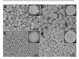
Figure 6. SEM images of intermediate products prepared with different in sources for various reaction times.  $In(NO_3)_3$  as In source for chalcopyrite CIS: 1 h (a), 3 h (b).  $InCl_3$  as In source for wurtzite CIS: 1 h (c), 3 h (d). The insets in (a), (b), (c) and (d) are the high-resolution SEM images of the products.
