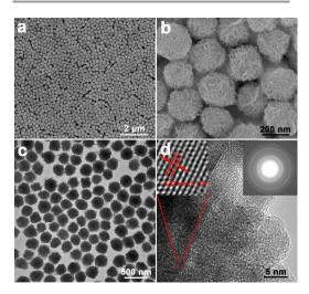
Figure 1. SEM (a and b), TEM (c), HRTEM (d and left inset) and SAED (right inset of d) images of the as-prepared CIS nanosoheres.
