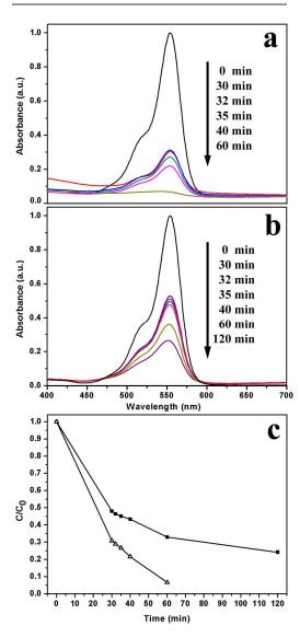
Figure 7. Temporal evolution of the absorption spectra of the aqueous RhB solution in the presence of chalcopyrite phase CIS (a) and wurtzite phase CIS (b) under visible-light irradiation. Photocatalytic degradation over RhB of CIS nanospheres (c). The triangles represent chalcopyrite phase CIS whereas the squares represent wurtzite phase CIS. The initial 30 min was stirring in dark for the adsorption equilibrium.
