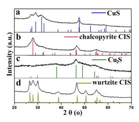
Figure 5. XRD patterns of intermediate products prepared with different In sources for various reaction times. In(NO<sub>3</sub>)<sub>3</sub> as In source for chalcopyrite CIS: 1 h (a), 3 h (b). InCl<sub>3</sub> as In source for wurtzite CIS: 1 h (c), 3 h (d). Reference patterns of CuS, Cu<sub>2</sub>S and chalcopyrite phase CIS from JCPDS cards are shown, along with a simulated diffraction pattern of wurtzite phase CIS.
