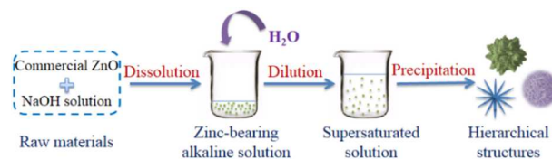
Fig. 1 Schematic illustration for preparation of ZnO hierarchical structures.
