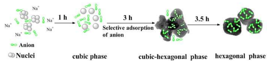
Fig. 5 Schematic diagram of crystal phase rapid transformation of NaYF 4 :Yb 3+ ,Er 3+ nanocrystals with the assistance of salts.
