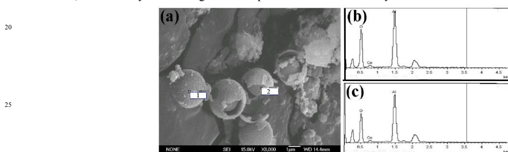
Fig. 2 SEM image (a), EDS spectrum of the shell (b) and the core (c) in the S-10 sample.
