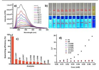
Fig. 2. a) The change in fluorescence intensity of compound **1** with incremental addition of PA. b) Digital photographs of solutions of compound **1** in the presence of different nitroaromatic analytes under normal light (top) and under portable UV light (bottom), c) The fluorescence quenching efficiencies of different analytes, d) Stern-Volmer plot for various nitro analytes.
